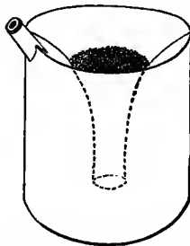
FIG. 107.—Counterpoise; weight when empty, 35 grammes; when full of dust shot, 200 grammes.
