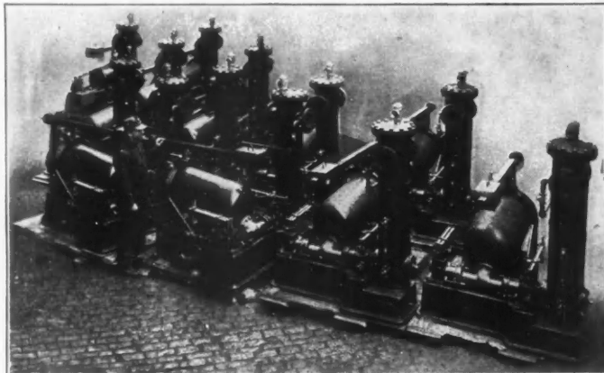
Group of 12 Crane Paper Machine Controllers.
