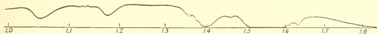
FIG. 3.—Energy transmission curve showing absorption spectrum of 5 cm. cell of liquid HCN at high dispersion. Slit width approx. 9\text{\AA} .
