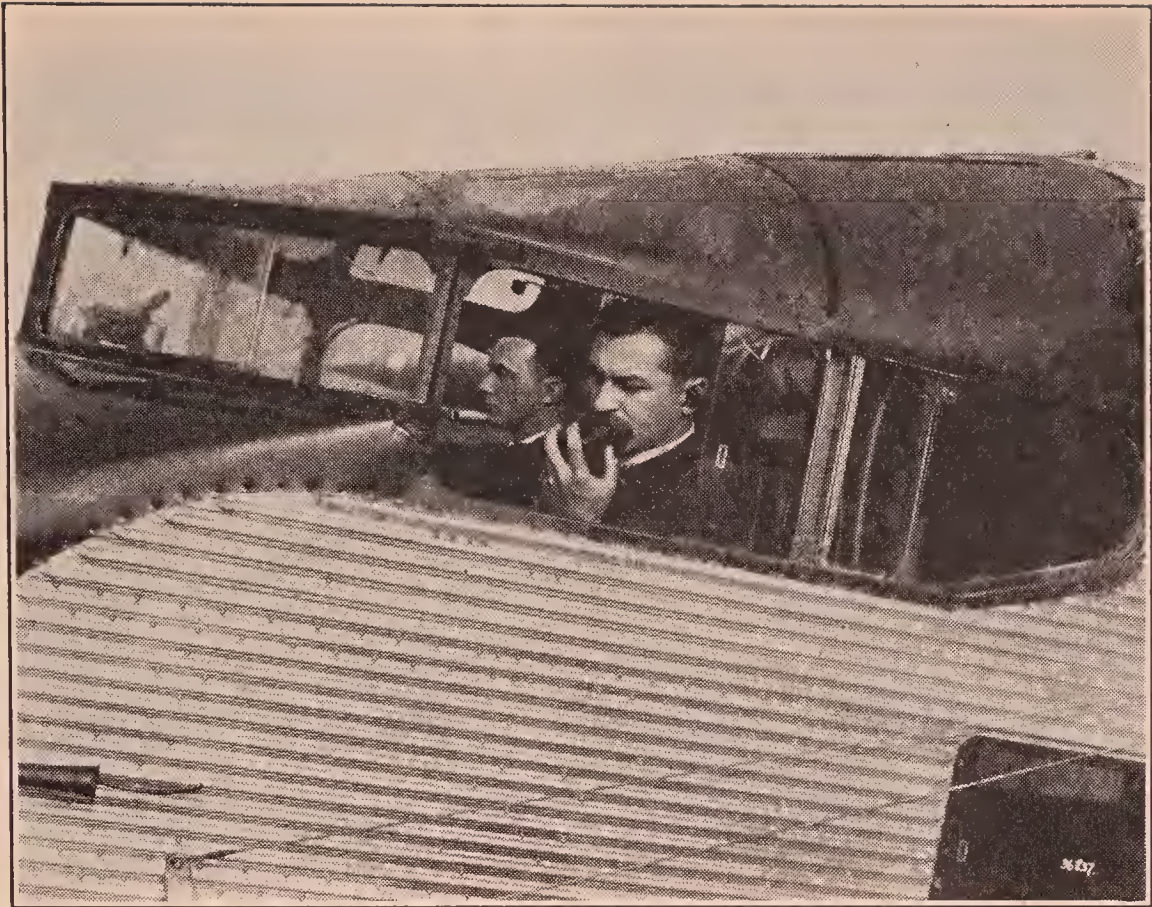
PILOT USING 'SILENCER' TYPE TRANSMITTER AND PHONETTE HEAD SET
