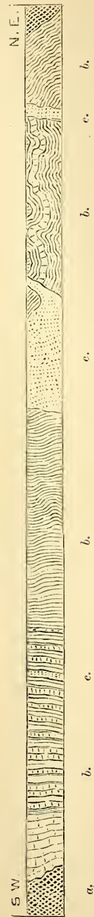
FIG. 2. SECTION OF TRIASSIC ROCKS, SECTION COVE, BURNABY ISLAND. a. Contemporaneous volcanic matter. b. Limestones and argillites. c. Dykes and intrusions. Scale, ten inches to one mile.
