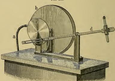
through the tube a, and removed by a similar tube not shown in the illustration. The water-wheel drives a circular metal disc c, in which, in one radius, is a series of holes. Into any of these holes is fixed a screw which connects the forked end of a long lever d to the apparatus. At the other end of the long piece d is a clamp for holding the test-tube, which is plugged when the apparatus is in motion.
