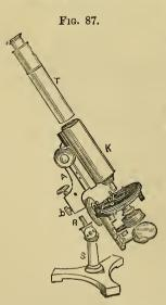
are used with artificial light), one of these lenses is removed and only one used, and a small secondary condenser placed under the stage of the Microscope. With this combination just described we can only project, with transmitted light, transparent objects.
