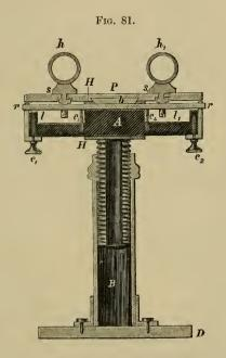
In a later form Dr. Blix has simplified the instrument, principally by the omission of the cylindrical axis A and the parts in connection with it.
