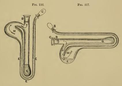
orifices are replugged, and then the gelatin melted by the aid of very gentle heat. The instrument is then placed in the horizontal position, fig. 117, so that the water and gelatin mix together in the bulb M. When thoroughly mixed, the fluid is dispersed over plates for the cultivation of this organism. The removal of the gelatin mixture is easily effected through the opening B.
