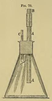
the way down the flask, and is closed at the outer end by a glass stopper B fitted on with a piece of indiarubber tubing. Into the other hole of the stopper is fitted the "exit tube" CC. This is a piece of glass tubing (1/4 in. diameter) bent round at the lower end, so that it opens in the neck of the flask just under the rubber stopper. It is open at both ends, but contains two cotton-wool plugs to prevent entrance of any micro-organisms from the outside.
