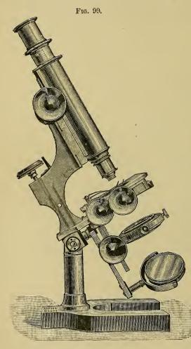
attached; it can be clamped by the screw in front. The substage has centering movements, rack-and-pinion coarse - adjustment, and differential - screw fine-adjustment, admitting of wide - angled condensers being easily focused. The usual plane and concave mirrors on a double-jointed arm are carried on an adjustable hinged tail-piece.
