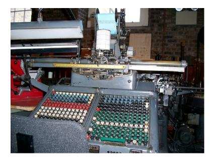
Figure 6.21: A keyboard for the Monotype casting system.
