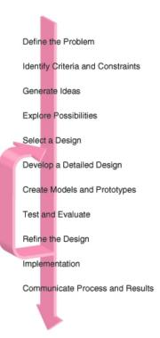
Figure 4.5: A spiral design process. Changes are made in the design, and then the improved design is evaluated.
