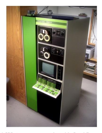
Figure 6.27: A PDP-12 minicomputer manufactured by Digital Equipment Corporation about 1970.
