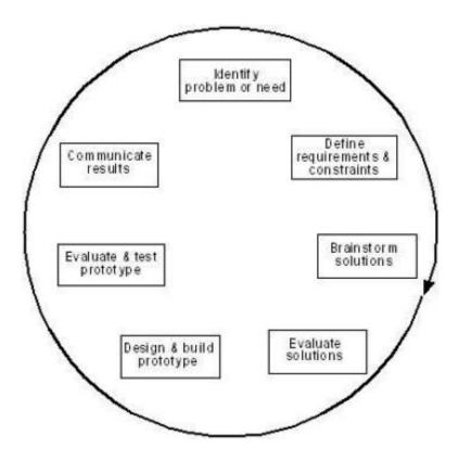
Figure 5.6: A simplified engineering design process.
