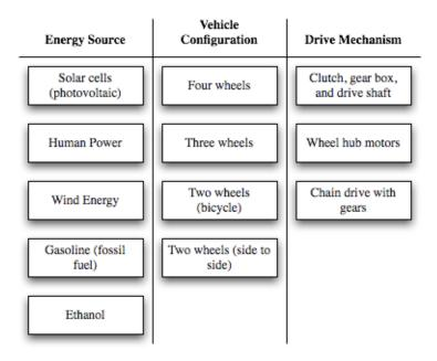
Figure 4.7: The concept combination table for the commuter vehicle.
