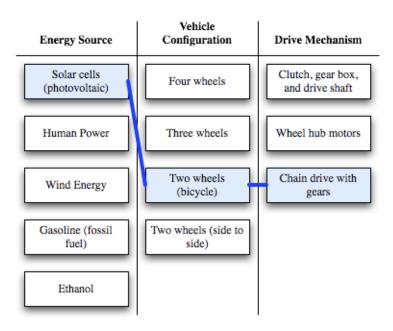
Figure 4.8: The concept combination table is used to generate a particular possible design.
