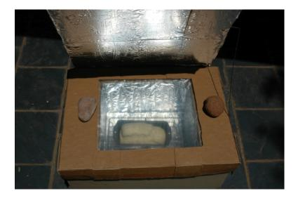
Figure 4.11: A simple solar oven made out of a cardboard box, foil, and clear plastic.
