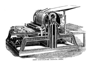
Figure 6.15: Rotary printing press invented by Richard Hoe.
