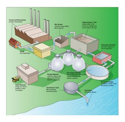
Figure 3.10: Steps in a typical was tewater treatment process.  $\,$
