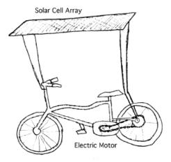
Figure 4.9: A sketch of the possible design obtained by from the concept combination table in Figure 16. Note that engineers often use rough, hand-drawn sketches at this point in the design process to understand design concepts and explore their strengths and weaknesses.
