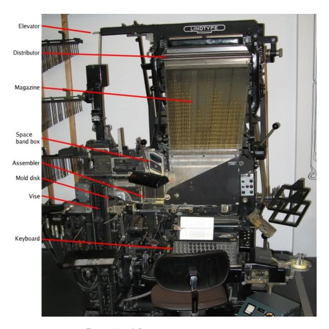
Figure 6.22: A Linotype type-casting system.
