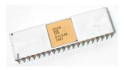
Figure 6.28: A Zilog Z80 microprocessor manufactured in 1976.
