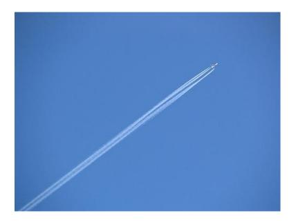
Figure 2.11: A high flying jet aircraft leaves contrails in the sky. A contrail is the white streak (or cloud) formed behind a high-flying aircraft's engines.
