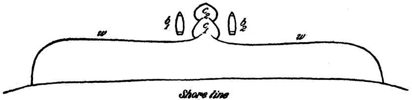
FIG. 3. Sabay, a transitory fish weir; diagrammatic. w , Wing; c 1 , c 2 , cribs or pounds; b 1 , b 2 , attending bancas.
