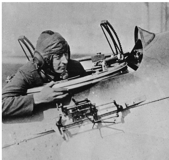
A Mk. I Drift Sight. The lever just in front of the bomb aimer's fingertips sets the altitude, the wheels near his knuckles set the wind and airspeed.
