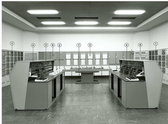
Layout of the Deltar. 1. Analog river sections 2. Peripheral equipment (Punched tape) 3. Operator controls 4. Measuring controls 5. Analog output (recorders) 6. Digital output (punched tape) 7. Design table (configuration of river setup) 8. Wind generator.
