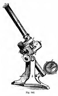
The powers are increased by a more powerful eyepiece or object-glass, or by both, or by lengthening the tube of the microscope.
