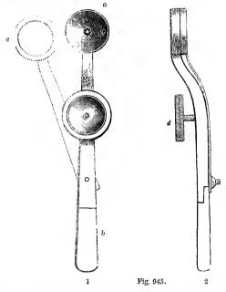
attached to a small brass handle (fig. 945, 1, b). For ordinary botanical purposes a lens magnifying 65 to 70 diameters is enough; but the lenses may be procured with a power of 150 to 220 diameters. On the plane side of this brass disc there is a ring of silver (fig. 945, 1, c), in which a thin piece of glass is fixed, also supported by a brass handle, which acts as a spring, so as to keep the two rings in contact.
