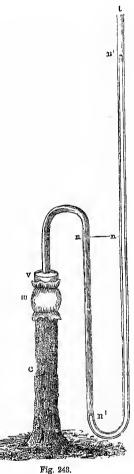
Fig. 243. Apparatus of Hales, to show the force of ascent of the sap. c, Stem of a vine cut. t. A glass tube with a double curvature attached to the upper part of the vine-stem, hy means of a copper cap, v, which is secured by means of a lute and piece of bladder. m. n n, Level of the column of mercury in the two portions of the tube at the commencement of the experiment. n n/, Level of the mercury at the conclusion of the experiment.
