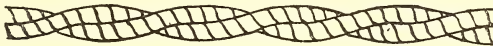
FIG. 4.—Two-ply Thread with Open-band Twist in the Singles and Cross-band Twist in the Double.
