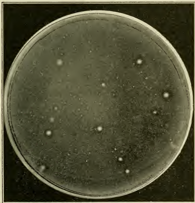
Agar Plate, showing colonies of bacteria in 1-500 eu. centimeter of effluent from Septic Tank.
