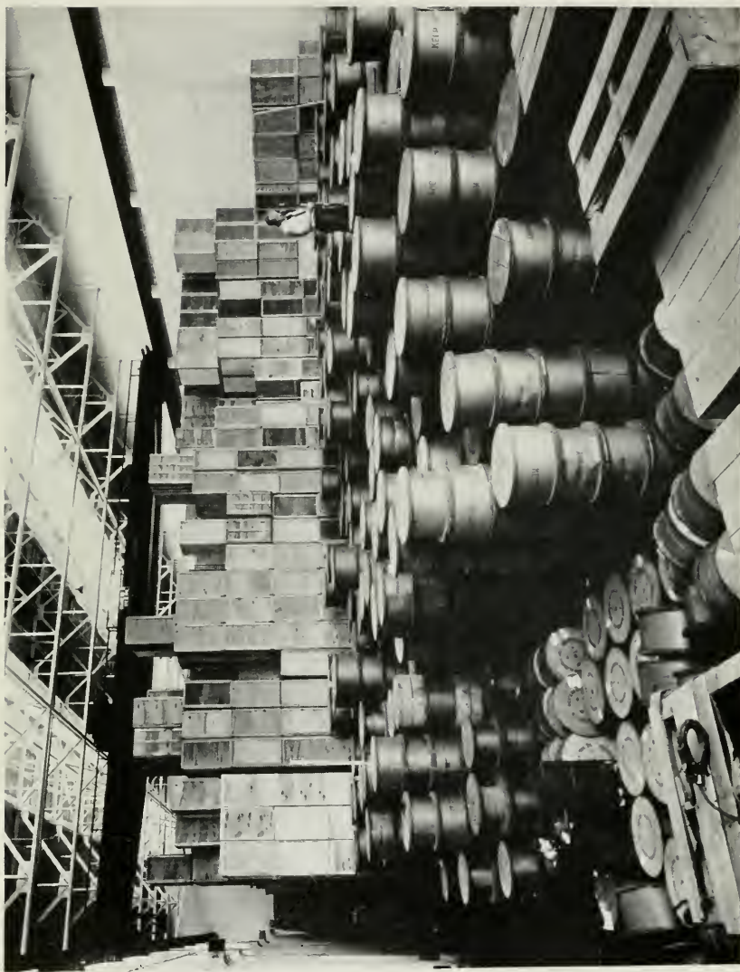
VIEW IN WAREHOUSE AT KEARNY, N. J., showing storage under cranes in building specially designed for that purpose.
