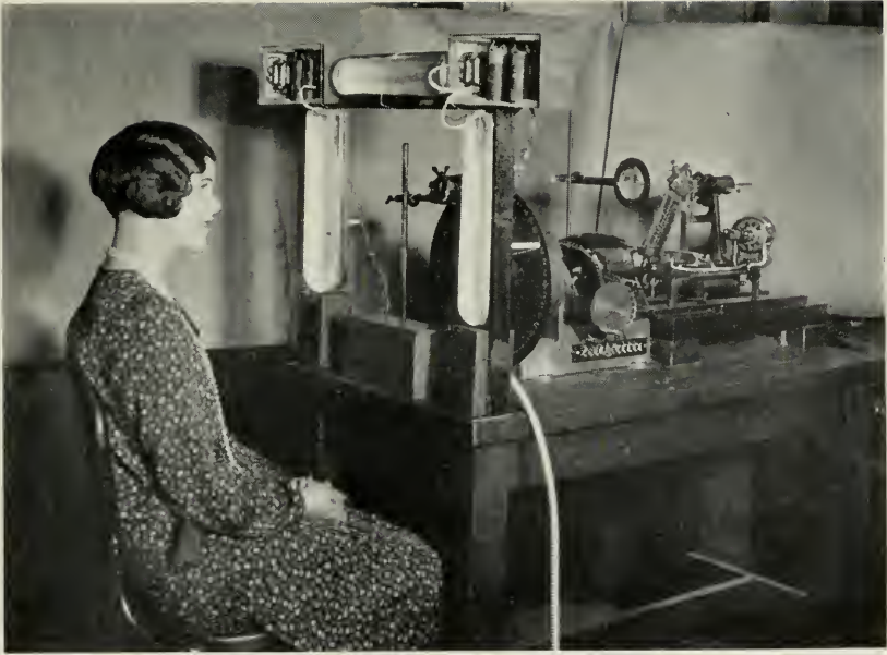
FIG. 8. APPARATUS USED AT THE SENDING END FOR TELEVISION.
