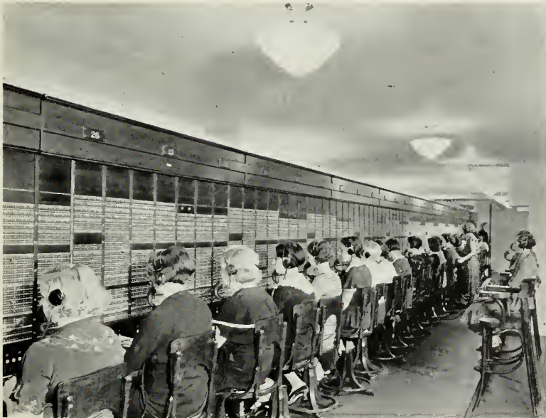
FIGURE 2. MANUAL SWITCHBOARD USED SEPARATELY.
