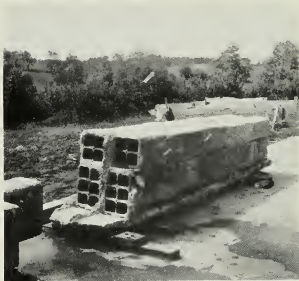
FIG. 4. MODIFIED STANDARD JOINTS WITH SUPPORTING BASE, AFTER TEST.
