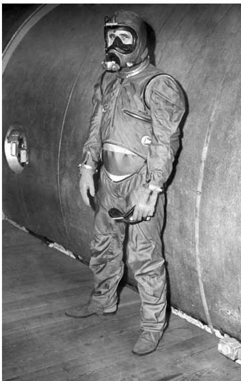
The Model 16 used a waist gusset that could be closed to control elongation while the pilot was seated or it could be opened to allow the pilot to stand erect as shown here. A pressure-sealing zipper running circumferentially around the chest just under the armpits allowed donning and doffing. The neck, shoulder, and wrist bearings were built into the restraint layer and were not part of the pressure bladder.
