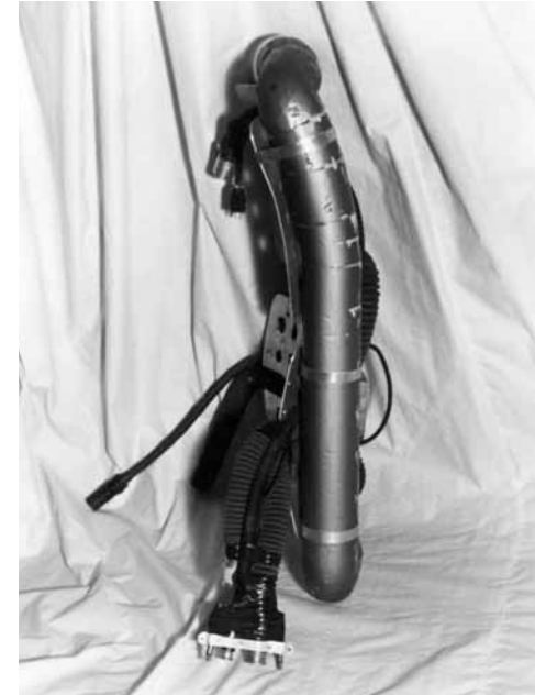
The Model 11 back kit was also an evolutionary improvement over the one used on the Model 7. Emergency oxygen was still carried in the outer frame, with the suit controller and breathing regulator in the center area. A standard parachute was worn over the back kit.
