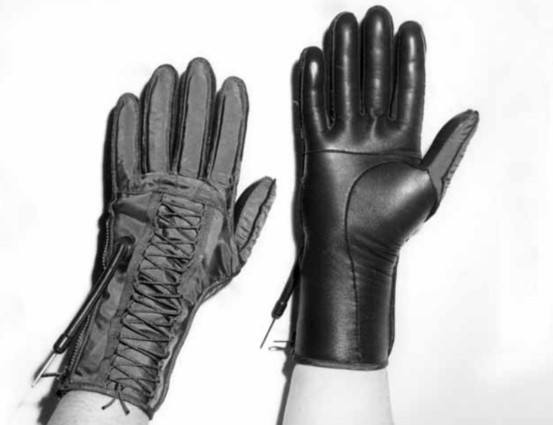
Above: David Clark Company S612 partial-pressure suit gloves were typical of the gloves used with later pressure suits. The gloves had leather palms and nylon backs. These particular gloves have the pressure lead on the pinky side; the MC-3 and MC-4 suit had pressure leads on the thumb side. Note the lace adjustments on the back.
