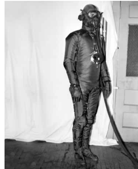
The Strato Equipment Company developed this Model 7 full-pressure suit for the U.S. Navy during 1947. Unlike most of the suits created for the Army Air Forces during World War II, most of the postwar suits developed for the Navy were fairly tight fitting.
