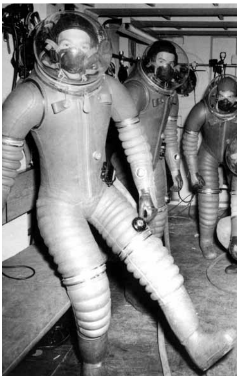
This photo shows at least four XH-5 suits in the Wright Field altitude chamber (only a part of the fourth suit may be seen at center right in a crouched position). Other photos from this series show six suits. The two suits nearest the camera are not fully pressurized, allowing the wearers to stand straighter than normal (note the hunched position of the suit at the back of the chamber).
