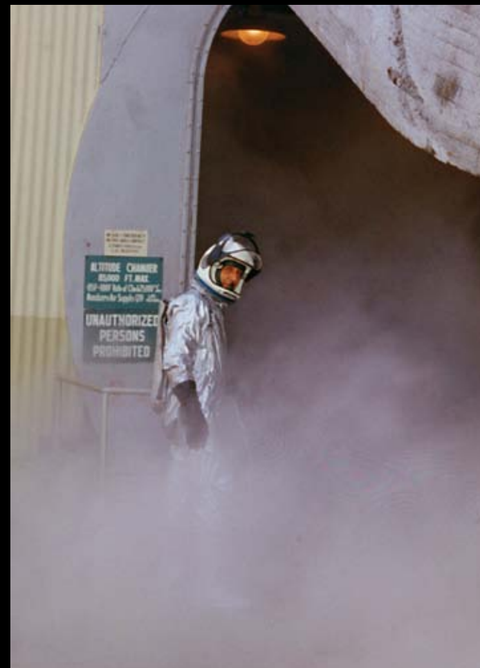
Another legendary test pilot, A. Scott Crossfield shows off an early David Clark Company MC-2 full-pressure suit in front of the Wright Field altitude chamber. The sign indicates the chamber was limited to 85,000 feet. Of note is the thickness of the raised entry door. – National Archives College Park Collection
