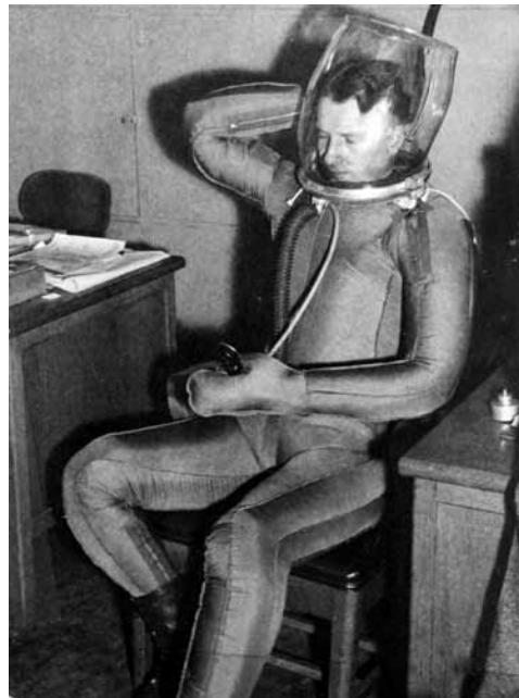
Dr. Kenneth Penrod, a consultant to David Clark Company, in the Experiment B suit. The unusual helmet showed up in several David Clark suits, as well as those from other companies. The suit allowed a fair amount of mobility, as demonstrated by Penrod holding his bended arm to touch the side of the helmet. Note the mittens instead of fingered gloves.
