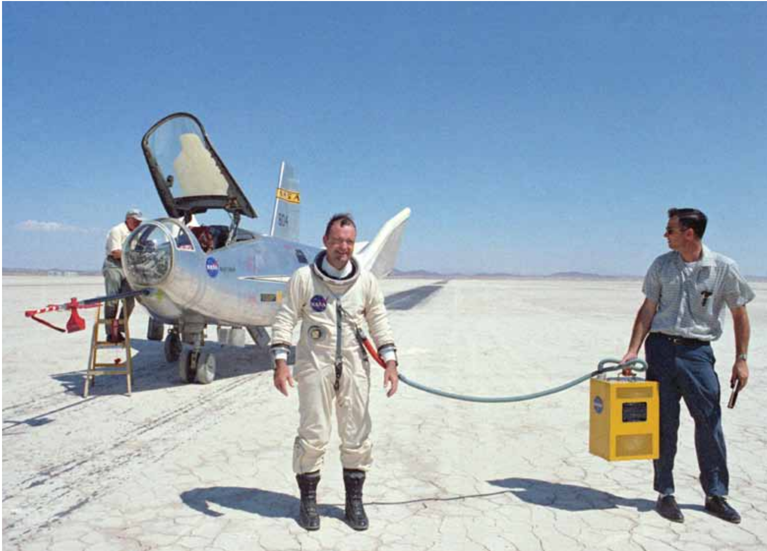
David Clark Company fabricated special versions of the AIP22S-2 for the NASA and Air Force lifting body programs. This is NASA test pilot William H. Dana standing in front of the HL-10 lifting body on one of the dry lakes at Edwards AFB, CA. Note the portable air-conditioning unit attached to the suit to keep Dana cool in the High Desert.
