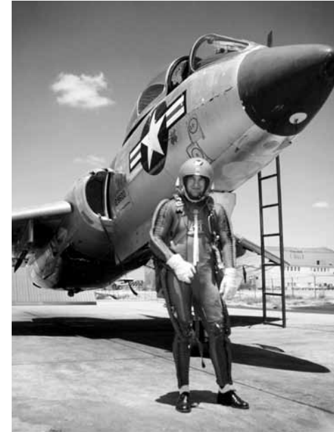
Chance Vought test pilot Jack Walton climbs into his F7U-3 Cutlass (BuNo 129600) wearing a David Clark Company C-4 partial-pressure suit. There is a parachute on his back, and an emergency oxygen bottle on his left leg.
