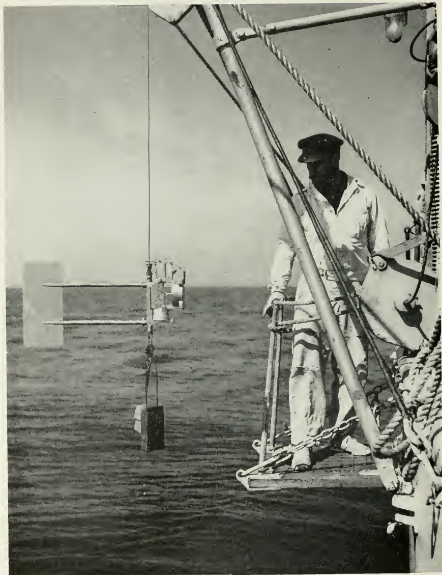
Currents are measured directly by means of specially designed meters, similar in principle to wind recorders, which are lowered on cables to the required depth. The fins ensure that the propeller which is turned by the current always faces toward it.
