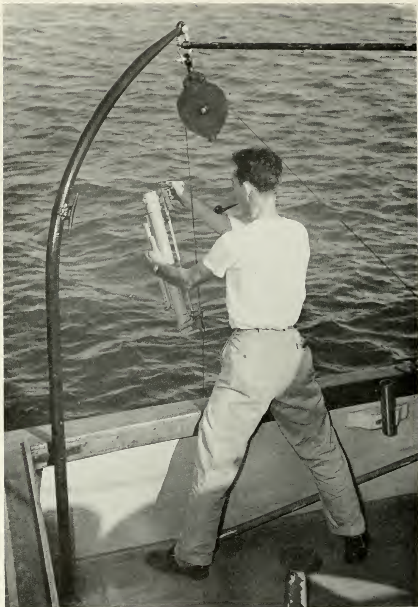
Samples of sea water used in the measurement of ocean currents are taken in special steel containers known as Nansen bottles. A series of these, open at each end, is lowered on a cable to the required depth. Weights are then sent down the cable which release one end of each bottle so that it turns upside down, at the same time closing each end so as to trap water from the required depths. Thermometers may be seen in metal tubes attached to the side of the bottles for measuring the temperature at each depth.
