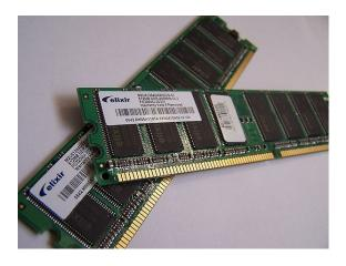
Example of writable volatile random-access memory: Synchronous Dynamic RAM modules, primarily used as main memory in personal computers, workstations, and servers.
