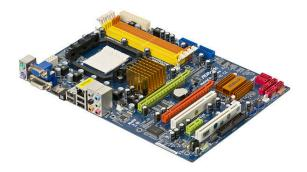
A motherboard with integrated graphics, which has HDMI, VGA and DVI outs.
