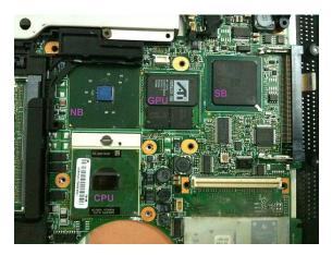
A part of an IBM T42 laptop motherboard. CPU: Central processing unit. NB: Northbridge. GPU: Graphics processing unit. SB: Southbridge.
