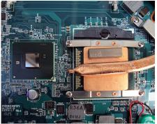
Intel Core i5 CPU on a Vaio E series laptop motherboard (on the right, beneath the heat pipe).
