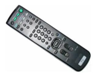
A typical firmware-controlled device: a television remote control. Consumer products like this have been using firmware since the 1970s.
