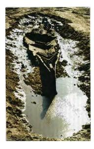
Plate 78 Wreck of a probable 19th-century double-ended carvel-built yawl or lugger with a central 'wet' hold, viewed from the stern, Mablethorpe, 1997
