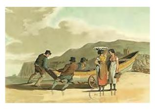
Plate 70 Earliest known accurate drawing of small coble being manoeuvred on a wheeled trolley, probably at Whitby, R & D Havell for 'Costumes of Yorkshire', 1814
