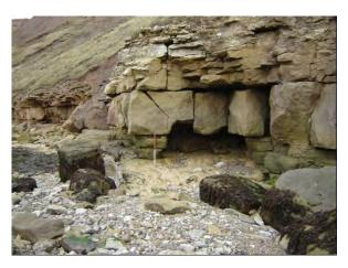
Plate 52 Pillar and stall quarrying, south side of Filey Brigg
