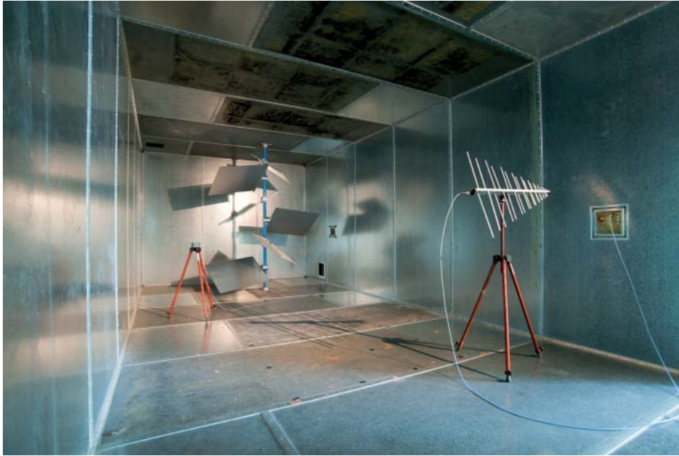
Figure 6. A mode stirred chamber, excited by a log-periodic antenna. (Source: Wikimedia Commons).
