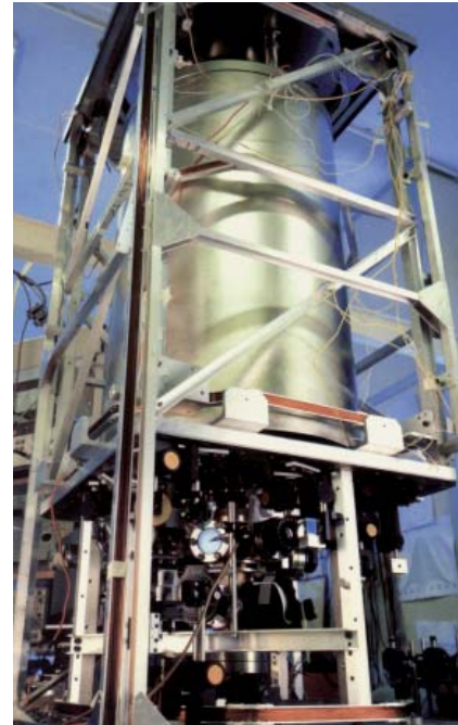
Figure 4. Cesium fountain clock FO-1 of LPTF, Paris (source: BNM-SYRTE, Observatoire de Paris).
