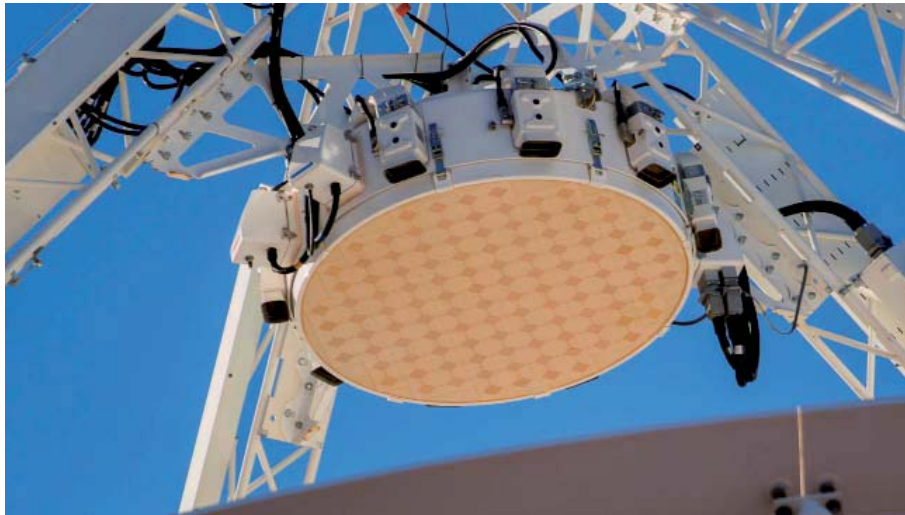
Figure 8b. A phased-array feed on an theASKAP antenna (credit: CSIRO).
