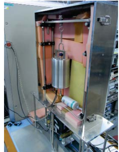
Figure 38. An RF power standard (calorimeter) for the frequency range from 220 to 330 GHz (photo by AIST).
