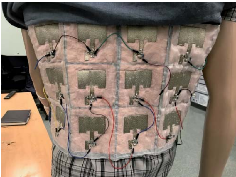
Figure 26. The antenna array with matching and harvesting circuits for woven electronic textile surface used for Wi-Fi energy harvesting (D. Vital, S. Bhardwaj, J. L. Volakis, “Textile Based Large Area RF-Power Harvesting System for Wearable Applications,” IEEE Trans. on Antennas and Propagation , 2020, https://ieeexplore.ieee.org/document/8883249 ).
