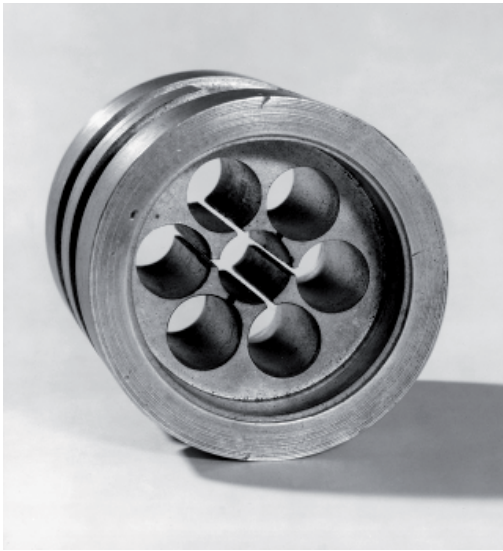
Figure 7. The anode block of the original cavity magnetron built in 1940 by Randal and Boot (from [13]).
