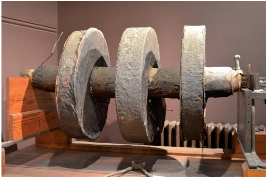
Figure 23. One of Callan's massive Induction Coils (1863), which produced voltages of 600kv and sparking gaps of 15 inches. (Credit: National Science Museum, St. Patrick's College, Maynooth, Ireland).
