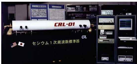
Figure 25. The optically pumped Cs PFS (CRL-01), which was jointly developed by NIST and NICT (CRL at that time) (photo by NICT).
