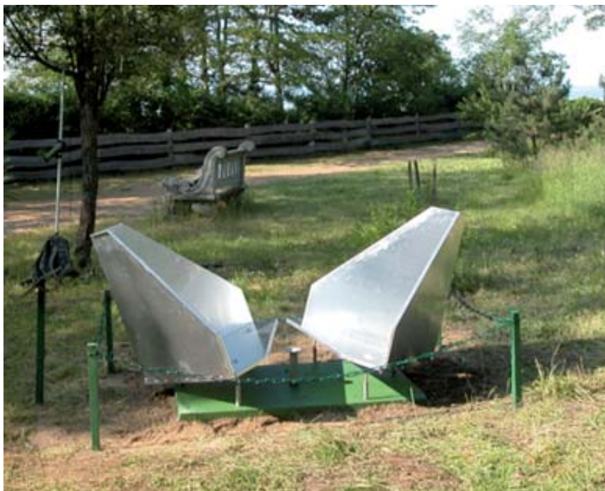
Figure 8. The manufactured face-to-face IBs for Sentinel-1 3D InSAR applications [16].
