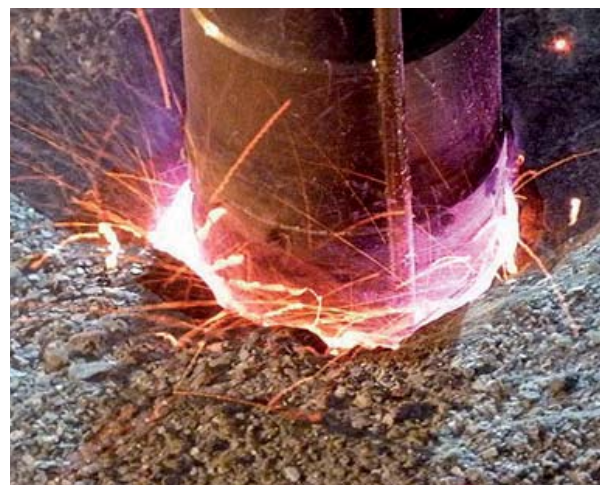
Figure 9. An illustration of Plasmabit and the plasma drilling process [34].
