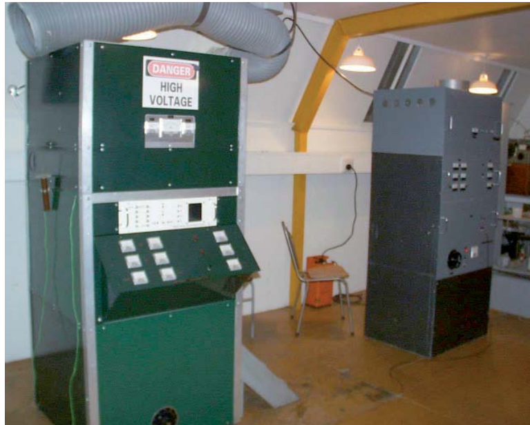
Figure 19. Meteor radar transmitters at the Birdlings Flat site (source: the University of Canterbury).
