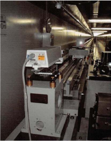
Figure 20. An interferometer for calibrating an optical distance meter (2001) [Section 8.1.1: 2]. This interferometer was installed in the tunnel for optical measurements (total length: 300 m) that was built on relocation to Tsukuba in 1979. It is an apparatus for direct calibration of an optical distance meter with the light wavelength standard as a reference using a 100 m traveling stage.
