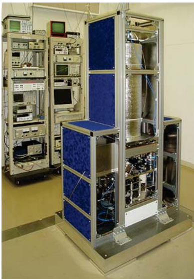
Figure 30. A cesium atomic fountain standard (2003). An atomic fountain frequency standard was developed in which laser-cooled cesium atoms are launched upward towards to a microwave cavity. Various factors causing frequency shifts were eliminated and the uncertainty of the primary frequency standard was reduced to the order of 10^{-15} (photo by AIST)
