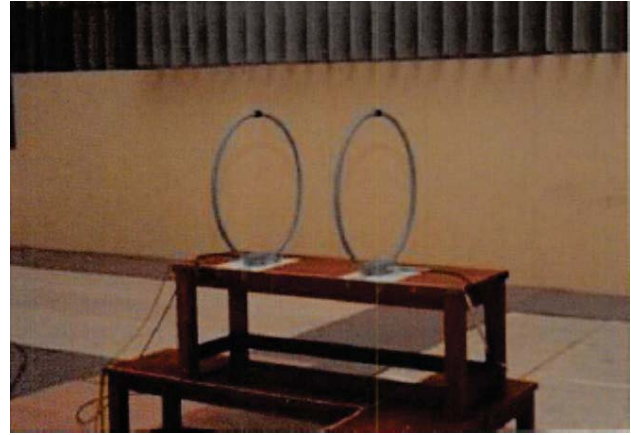
Figure 28. Preparation of loop and monopole antenna in the long-wave region (2002) [Section 8.1.1: 2]. Antenna factors of loop antennas are measured using the three-antenna method as a standard antenna on magnetic field below 30 MHz. The institute participated in the international comparison held in 2002.
