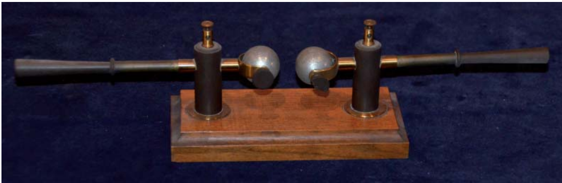
Figure 5. The spark gap-rig used by Marconi on board the Flying Huntress, Dublin, 21 July 1898. (Credit: National Science Museum, St. Patrick's College, Maynooth, Ireland).
