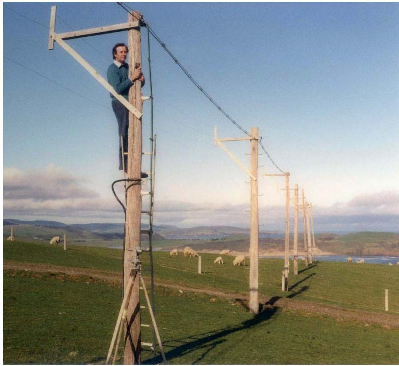
Figure 9. The 55.3 MHz co-linear array for the Slope Point auroral radar (with Paul Johnston) ~ 1970 (source: DSIR).
