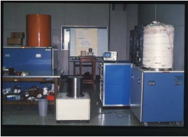
Figure 17. The left and right systems are sequentially developed hydrogen masers. The center system is a compact hydrogen maser developed as an engineering model for a quasi-zenith satellite. This photo was taken in 1990 [Section 8.1.1: 1].
