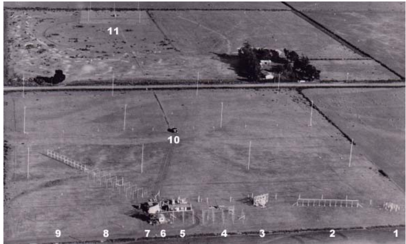
Figure 14. The layout of the Rolleston Field Station ~ 1960 (source: the University of Canterbury). Key: (1) Omnidirectional crossed dipoles for all-sky meteor radiant survey; (2) Broadside array for meteor radiant determination; (3) Broadside rotating (360 deg) array (first installed 1951); (4) Eight Yagi antennas for meteor radiant determination; (5) Receiver and recording building for 69 MHz; (6) COL 200 MHz radar originally at Wigram RNZAF base; (7) Housing for the 69 MHz GL Mk 2 transmitter; (8) Yagis for meteor radiant determination; (9) Broadside array for meteor radiants; (10) Broadside 1.75 MHz TX array for partial reflection radar; (11) The 1.75 MHz circular polarisation receiving array.
