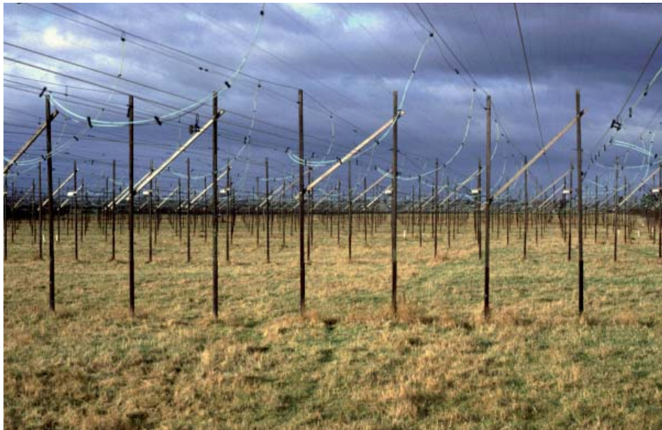
Figure 12. The IPS Array for investigating interplanetary scintillation, used to discover pulsars (credit Graham Woan, University of Glasgow).
