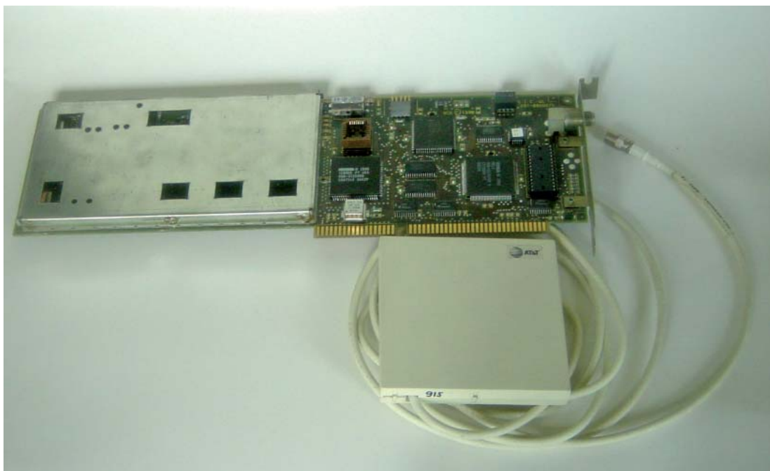
Figure 6. The first prototype of a WaveLAN card (image courtesy of Vic Hayes).
