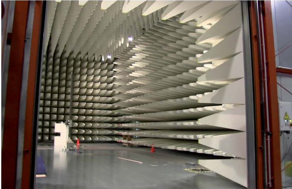
Figure 3. A log periodic antenna illuminating the EUT in an Anechoic chamber. (Source: Wikimedia Commons).
