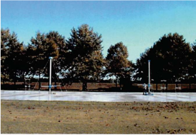
Figure 27. Preparation of the antenna factor standard for dipole antennas (2002) [Section 8.1.1: 2]. An open-area test site for the frequency range of 30–1000 MHz. Antenna properties are determined by measuring the propagation attenuation between two dipole antennas set up on the ground plane. The institute participated in an international comparison in 2002.
