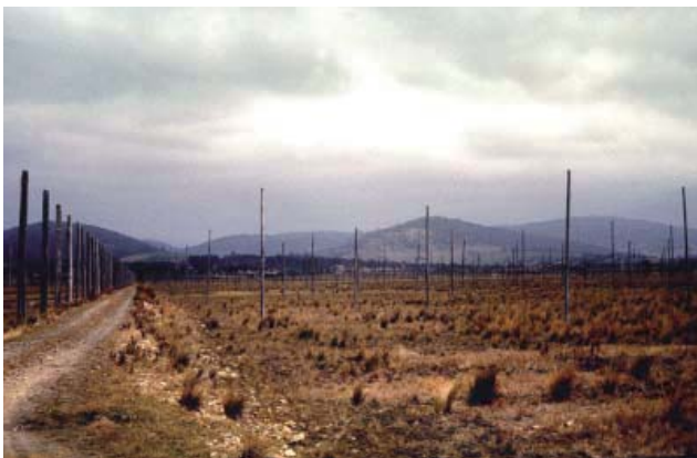
Figure 7a. The poles of the Llanherne Low Frequency Array near Hobart, Tasmania, operating at frequencies between 2 MHz and 35 MHz. This was one of the University of Tasmania's major low-frequency instruments. It was used from 1972 to the early 1980s to record decametric bursts from Jupiter and to map the radio sky at low frequencies [46] (credit: the estate of Grote Reber)
