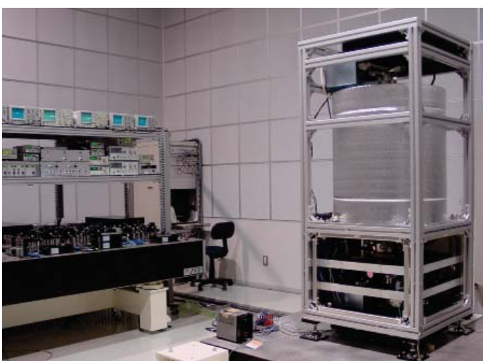
Figure 32. The cesium atomic fountain primary frequency standard NICT-CsF1 (photo by NICT).
