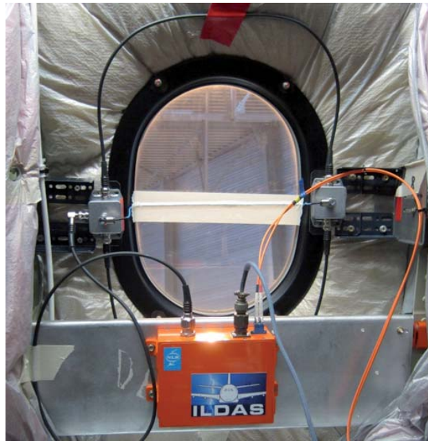
Figure 9. A window sensor for the lightning magnetic field, considered as a thick slotted antenna. In the setup shown the flux capturing area is of the order of a^2 where a is the long axis of the window for a horizontal current density in the fuselage. With the wire vertical, it is sensitive to a vertical current density, although with different sensitivity.
