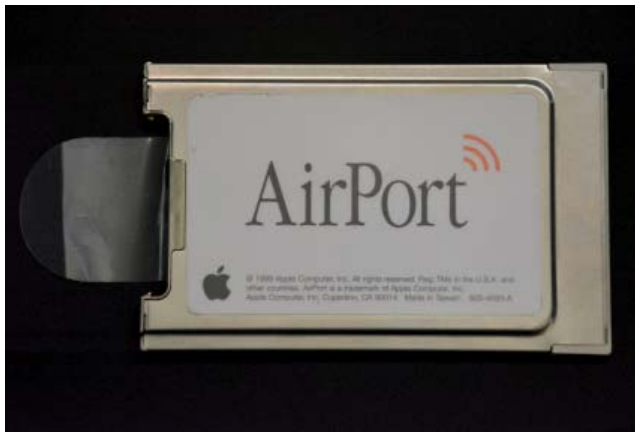
Figure 7. The Wi-Fi card in the 1997 Apple MacBook (left, image courtesy of Vic Hayes and Frans Florentinus) and the Apple Radio Access Point (RAP, right, image courtesy of Vic Hayes).
