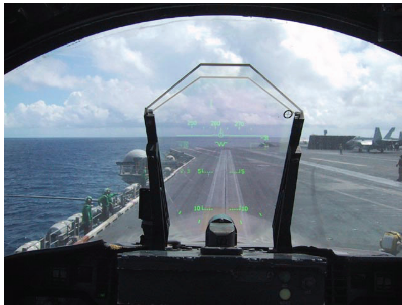
Figure 3-12. Example of head-up display (HUD) in F/A-18C (National Aeronautics and Space Administration).
