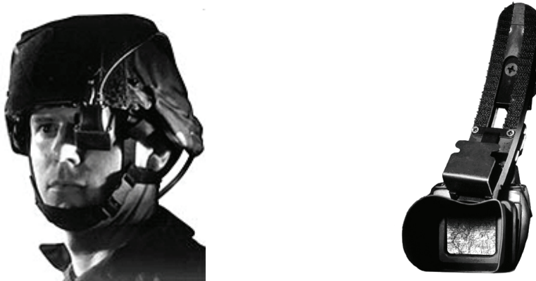
Figure 3-30. The Land Warrior HMD concept and the Rockwell Collins ProView™ S0-35 (Rockwell-Collins, 2008b).
