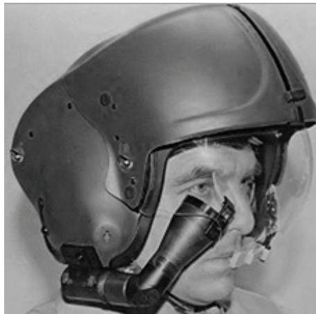
Figure 3-9. Integrated Helmet and Display Sight System (IHADSS).
