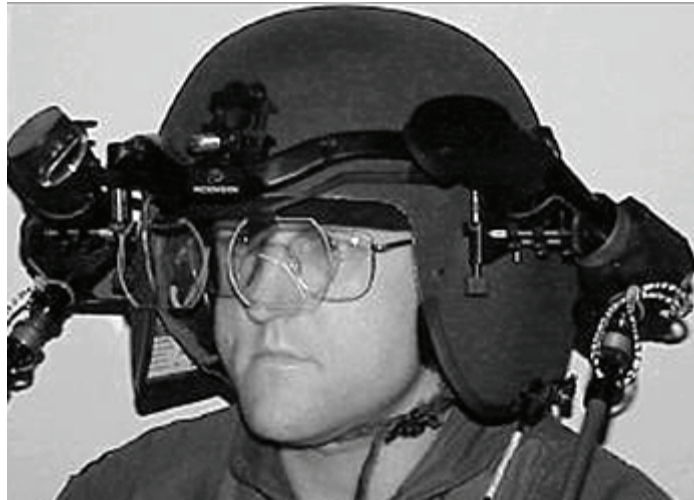
Figure 3-26. Prototype AIHS scanning laser HMD (Microvision, Inc.).
