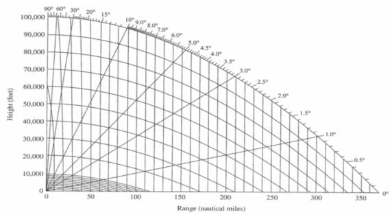
Radar range-angle-diagram used to plot antenna coverage, based on exponential model of refraction with = 313.
