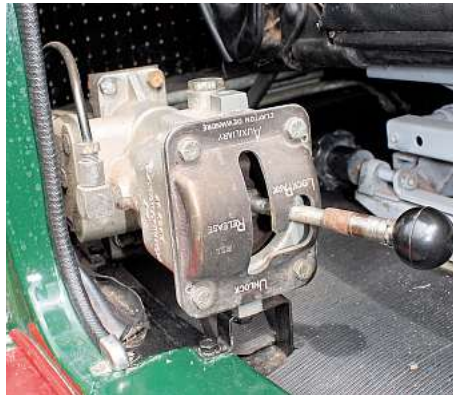
The lock actuators for the handbrake system. I've never been a fan but Graham says he could drive the lorry and use the handbrake – a bit – to dab the brakes on. Saved using his foot – I've never heard of that before.
