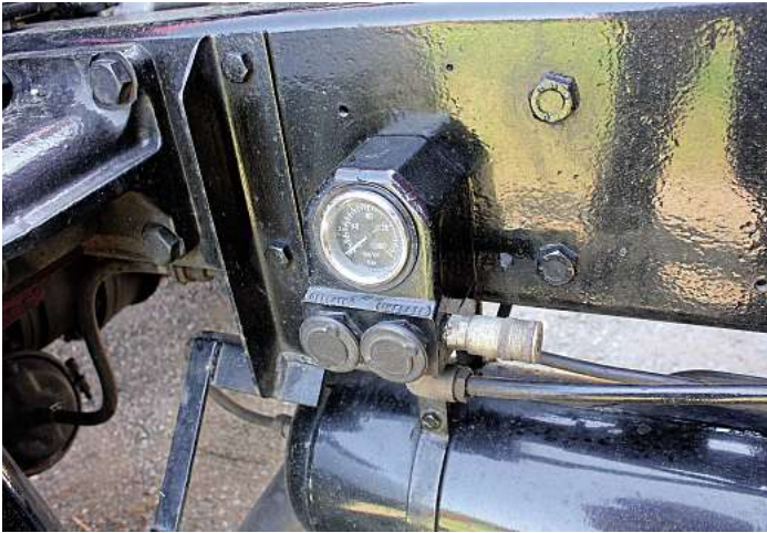
Scammell always fitted these tyre inflators behind the cab on the chassis.
