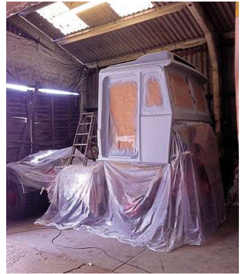
The Foden was purchased with a seized Cummins 250 engine and a worn out diff. The cab also required major work due to cracked glass fibre panels and rotten timber framing.
