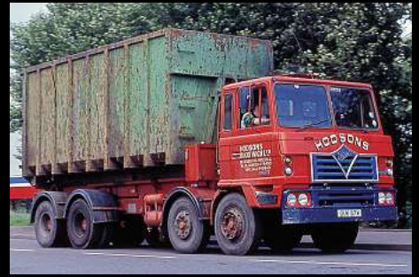
North of Walsall in a district called Bloxwich is a fairly large scrap metal merchants called Hodsons. It has used ERFs over the years but an equal number of Fodens, most of which had roll-on/roll-off bodies like this Haulmaster taken in June 1990.
