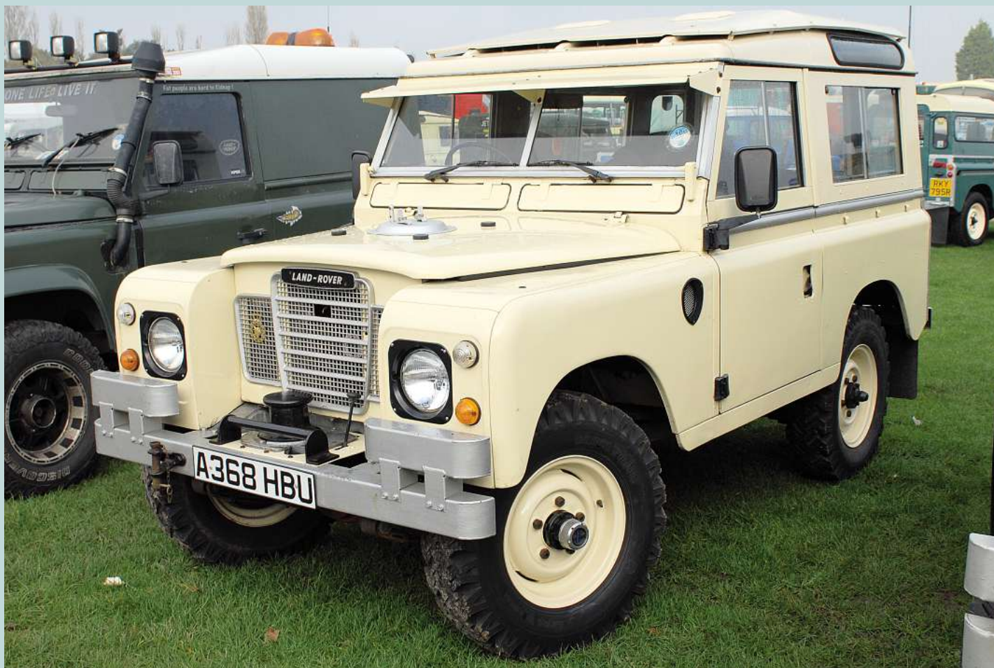
A well looked after 88in example with freewheeling hubs, sun visor, Safari double-skinned roof, capstan winch and military 'bumperettes'. Note the heater intake vent on the front nearside wing.
