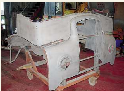
Work under way. Jamie describes the cab as in a terrible state and only held together by its paint!
