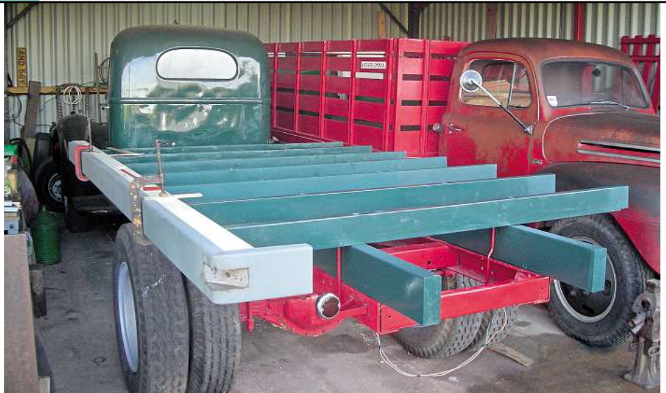
Body construction. Mike ordered new ash timber cut to size but when it arrived it was unusable so was replaced with pine and oak.
