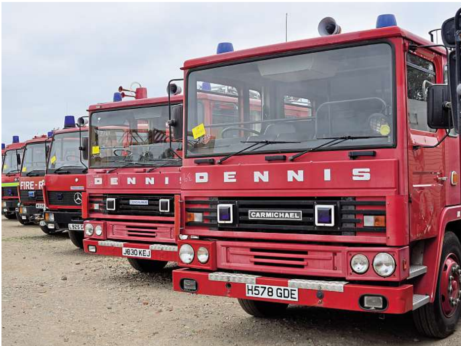
Local authority fire engines find their way here too. A quantity of the Norfolk brigade's Mercedes-Benz 1124 machines, with Saxon equipment, finish a line started by a pair of Dennis SS239 machines, one with Carmichael (H578 GDE) and the other Excalibur (J830 KEJ) bodies. £5500 is the suggested price.
