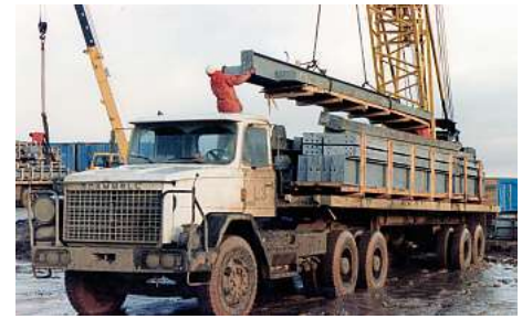
The Scammell's fifth wheel required alterations to allow it to couple to the 40ft flats.
