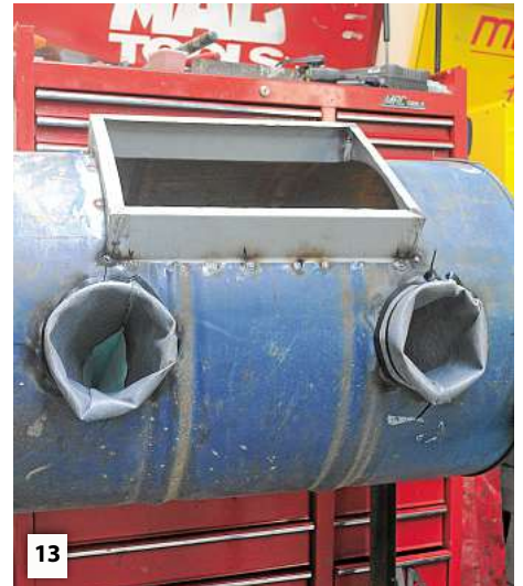
13 Both gloves were now fitted, and tested for length etc.
