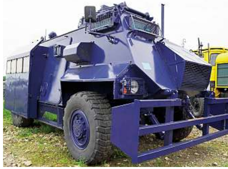
A GKN-Sankey AT 105 Saxon riot vehicle displays its hydraulically-operated crash-bars and side-protection wings.
