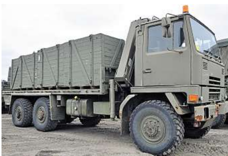
One of the final 6x6 Bedford TM 14-16 tonners to come through. It's especially rare as this is a CALM truck, (Crane, Lorry Mounted) loading crane, two-ton.
