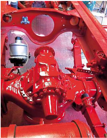
The Foden was purchased with a seized Cummins 250 engine and a worn out diff. The cab also required major work due to cracked glass fibre panels and rotten timber framing.
