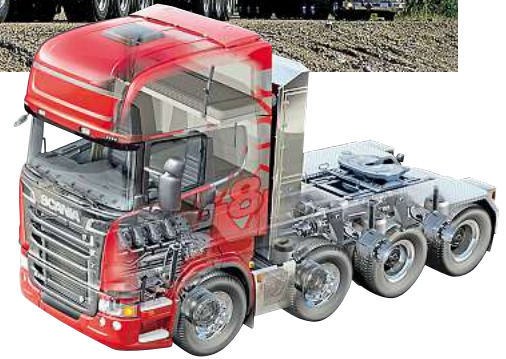
Today's Scania range-topper is the 730bhp R730 8x4 heavy haulage tractor. Rated gross combination weight is 250 tonnes.
