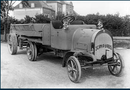
This 1914 type CLC with what looks like an adapted horse wagon trailer must have been one of the world's first artics.
