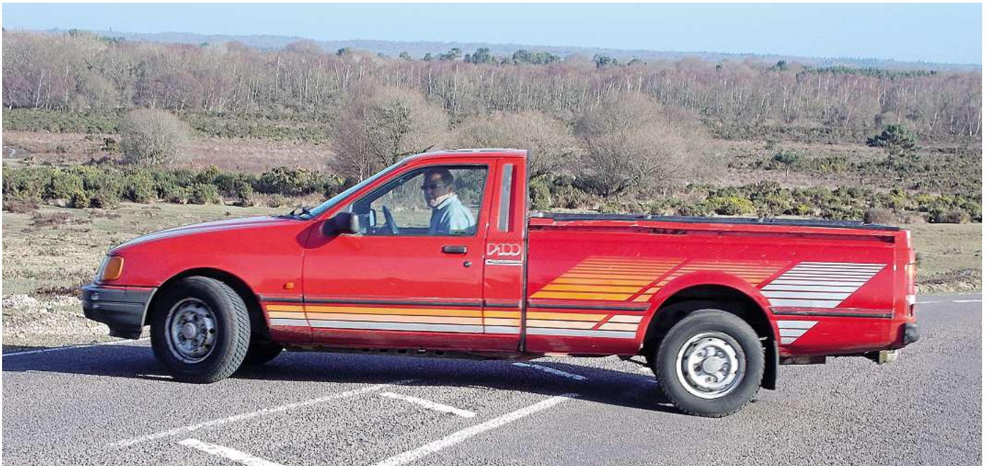
The P100 was very different to the Sierra car. Differences include a separate chassis, different gearbox and rear axle, and Ford Transit wheels.
