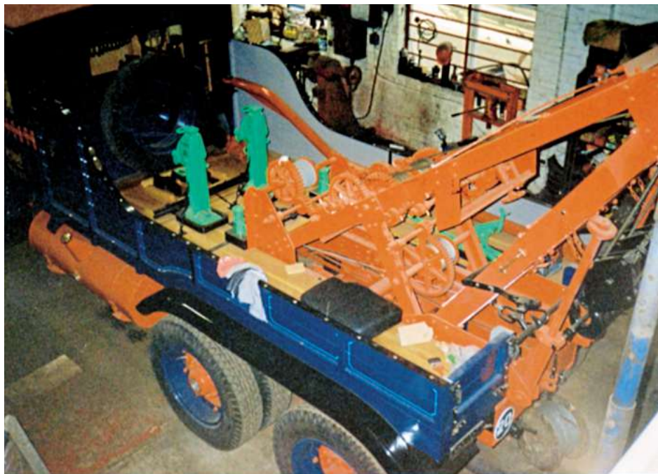
Fitting the Harvey Frost twin boom eight-ton crane.
