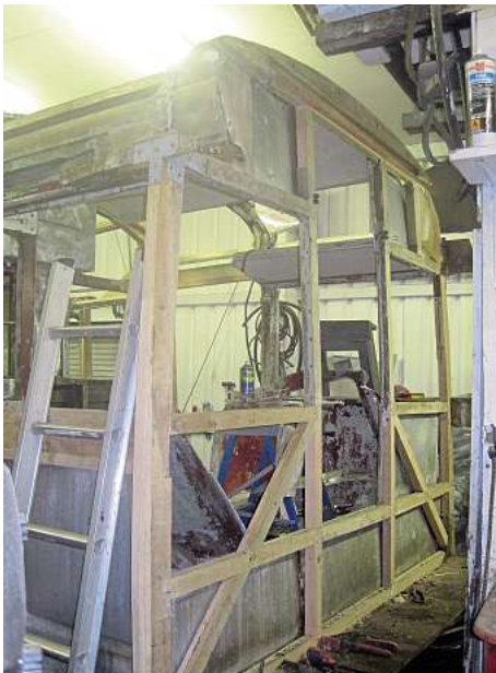
The wooden body frame was completely rebuilt using new ash and mahogany.
