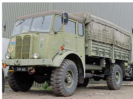
The ultimate gun-towing vehicle? A 'Matamillydor', an AEC Militant Mk2 cab, grafted on to a Matador chassis. What might have been!
