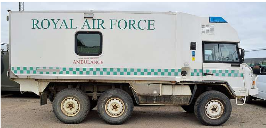
The Steyr-Puch Pinzgauer, model 7718 and RHD, this is the ambulance version supplied to the RAF.
