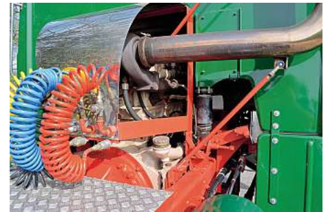
The seized engine was replaced with a 14 litre 350 Cummins. As this came from an American vehicle it had 12 volt electrics which have been changed for a 24 volt system.
