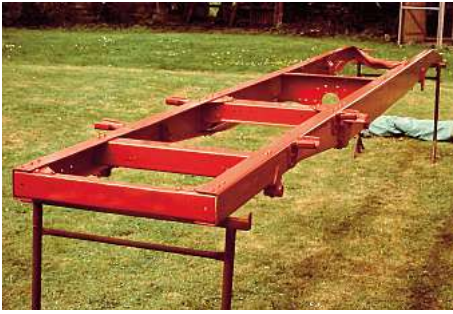
The truck was completely stripped and the chassis shot blasted and painted.
