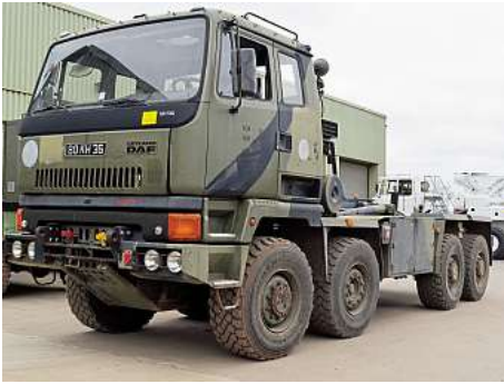
80 KH 36, the four-axle DROPS big hook, now given some chunky tyres, 8x6 drive and branded Leyland DAF.
