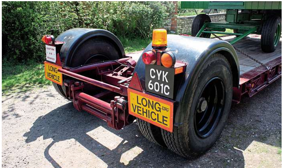
The rear of Tasker trailer can be pulled away by one person – Nick says – after jacking it up, removing lines etc.
