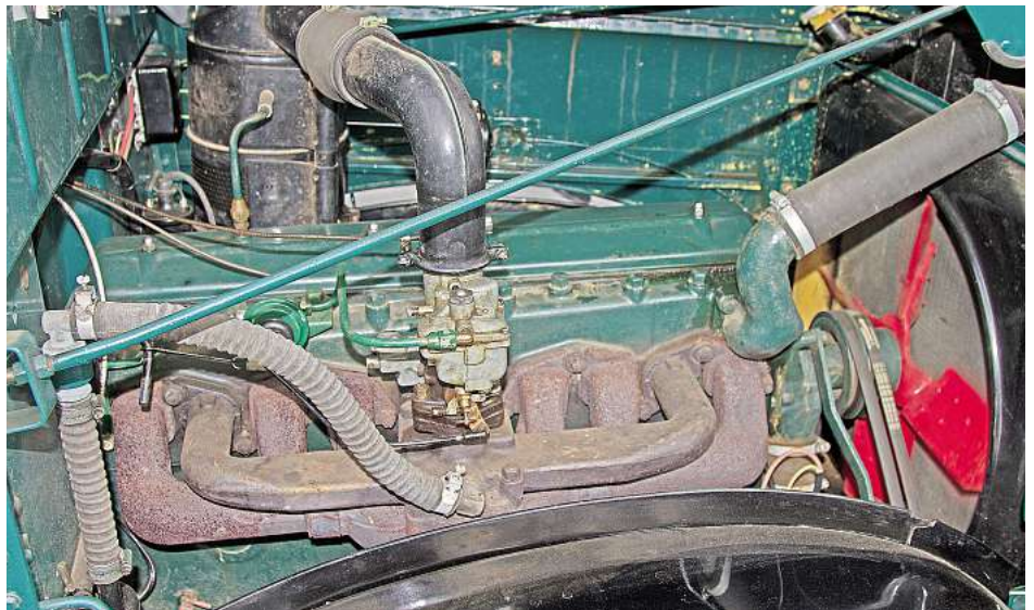
The 521cc overhead valve straight-six petrol engine.
