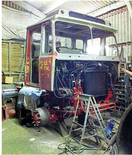
The Foden was purchased with a seized Cummins 250 engine and a worn out diff. The cab also required major work due to cracked glass fibre panels and rotten timber framing.
