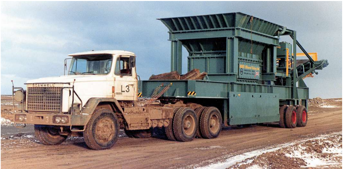
The S24 moving one of the stone crushing plants.
