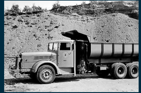
The long bonnet of this Scania-Vabis 10-tonner of 1941 houses a straight-eight. The tank behind the cab indicates it ran on producer gas.
