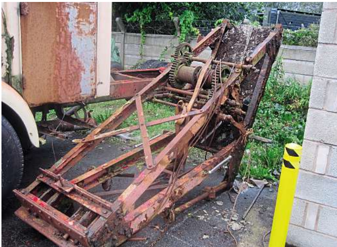
The hand cranked Harvey Frost crane would be refurbished by the Belle Vue Coach Company's apprentice mechanics.
