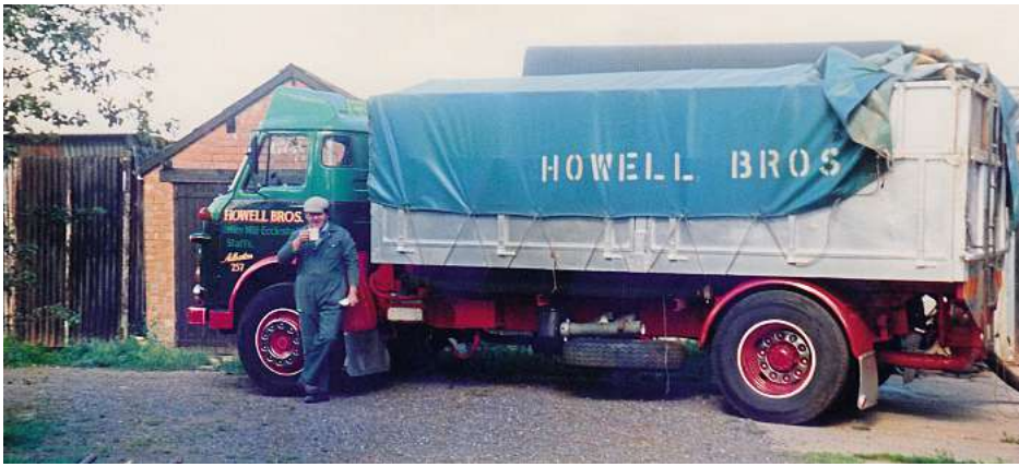
The lorry in its working days, and Graham has a cup of tea as he unloads with the blower. It might take half an hour to unload – in blower form it carried about 9.6 tons.
