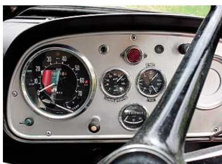
Note the air blower gauge that's related to the engine's supercharger.
