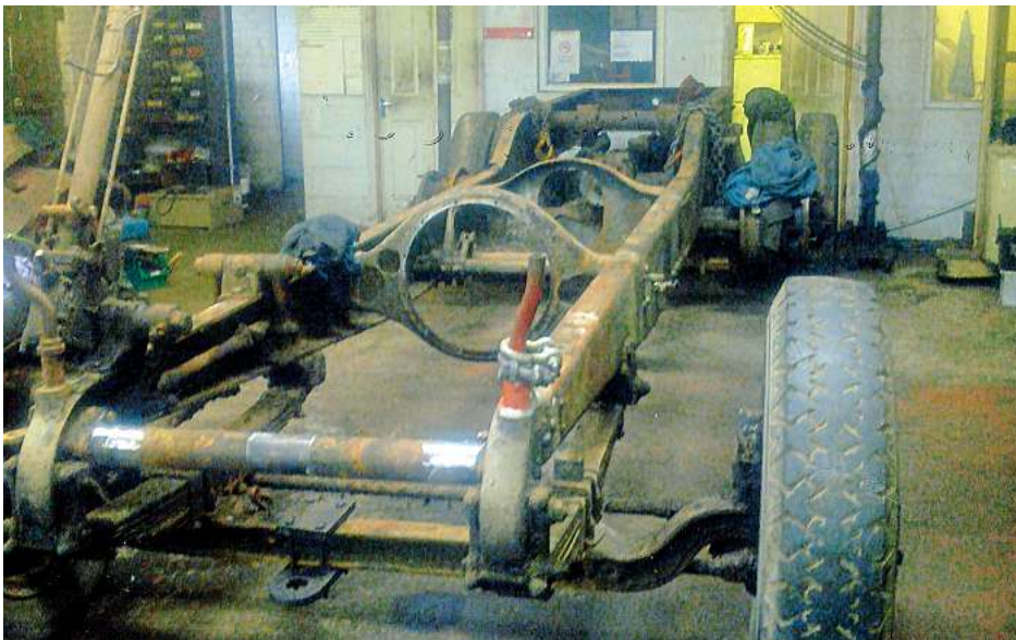
Stripped to the chassis. Virtually every moving part was seized.
