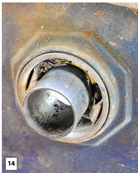
14 The main barrel bung was placed at the top of the sandblast cabinet; a piece of exhaust pipe was brazed into a hole cut in the bung for dust extraction using a wet and dry vacuum cleaner.
