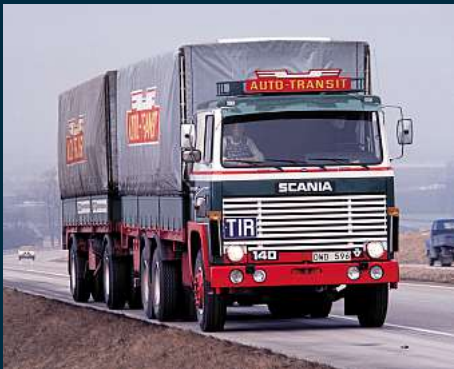
The LBS140, with a 14-litre V8 turbodiesel producing 350bhp, was the most powerful volume-built truck in Europe when it debuted in 1969.
