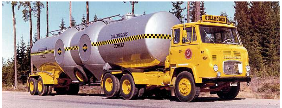
The LB76 was part of the line-up launched in 1963, when Scania-Vabis moved into the forward-control market after switching exclusively to bonneted trucks a quarter of a century previously.
