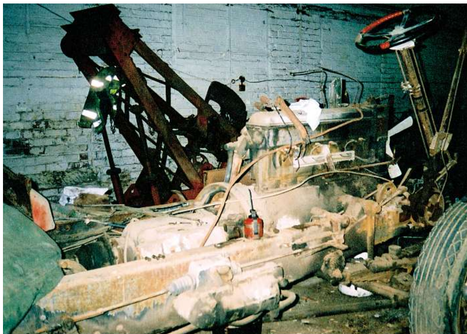
The six-cylinder petrol engine was in remarkably good condition. With the oil changed and filters, plugs and leads cleaned, it was soon ticking over nicely.
