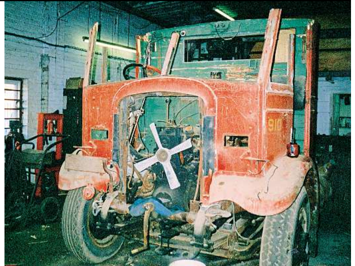
The cab and on-board workshop were traditionally rebuilt with an ash frame and walnut for the workshop floor.
