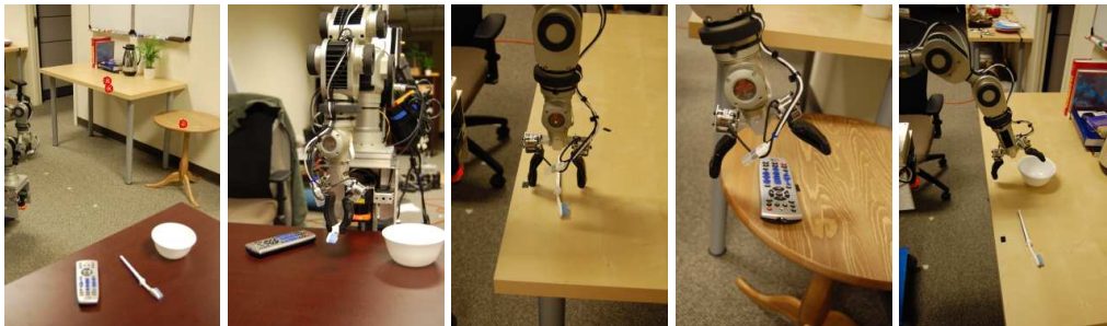
Fig. 14: (Color online) This figure shows the object placement experiment. The first image shows the three objects (TV remote, toothbrush and bowl) and the desired placement points (red circles). The second image shows the robot grasping the toothbrush, and the remaining three images show the robot placing the toothbrush, the TV remote, and the bowl.
