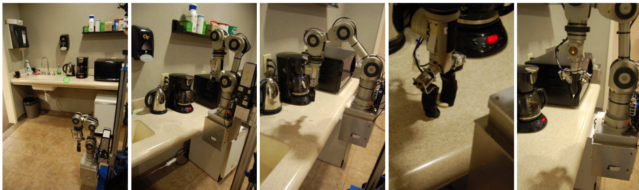
Fig. 4: These images are from one of the experiments that we performed to evaluate the performance of the robot (Section 5.1). The robot picks up a pill from a kitchen counter top after the user briefly illuminates the pill with a laser pointer. The first image shows the starting location of the robot. The robot approaches the pill in a direction normal to the surface, segments the pill and positions the gripper above the pill. The gripper then moves down until it makes contact with the surface and picks up the pill.
