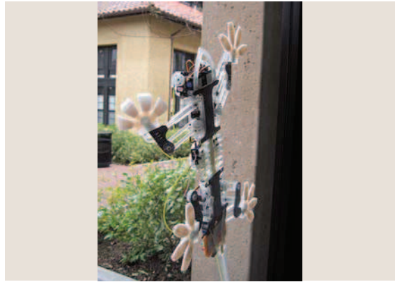
Fig. 60.12 Stickybot, the artificial gecko ©Mark R. Cutkosky, Stanford University Center for Design Research
