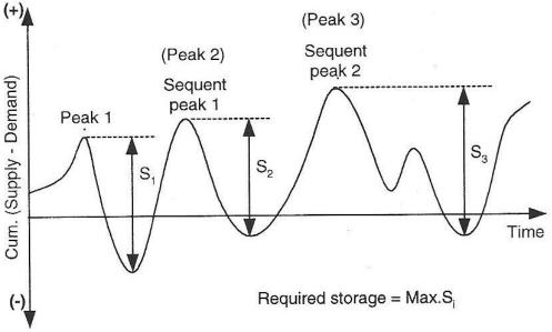
**4.** The storage required between these two points is the difference between the first peak and the lowest point in this period.
