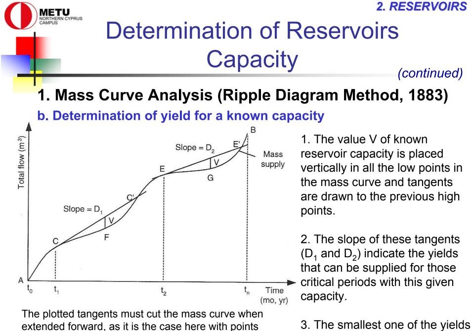
extended forward, as it is the case here with points C' and E'. Otherwise, the reservoir will not refill.
