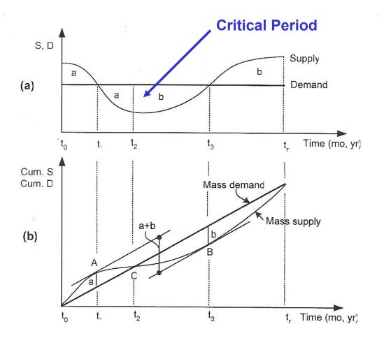
Required storage capacity of the reservoir is the vertical difference a+b
