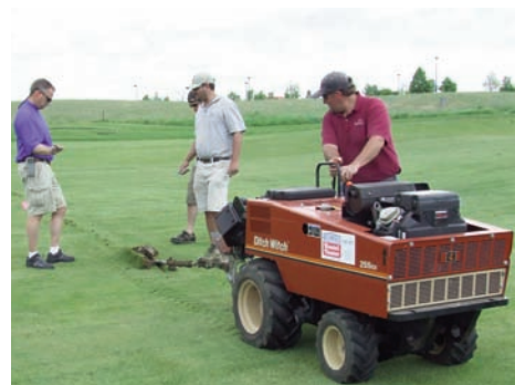
A total of 12 sensors were installed on each fairway to measure temperature, volumetric water content, and electrical conductivity of the soil.
