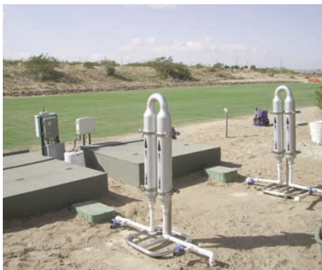
Conditioning treatments included two catalytic water conditioners (Zetacore and FreFlo), a magnetic water conditioner (Magnawet), a hydro-electrical conditioner (Aqua-PhyD), and a control treatment.
