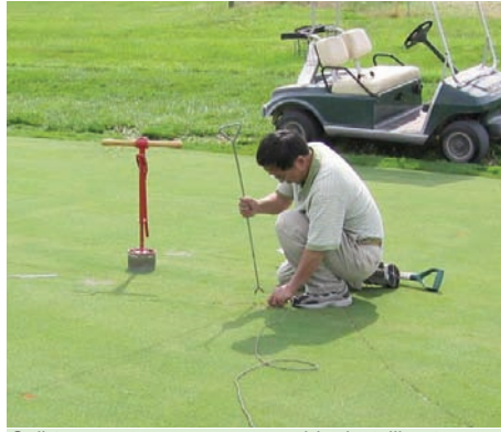
Soil temperature was measured by installing temperature sensors about 0.8 inches below the soil surface.
