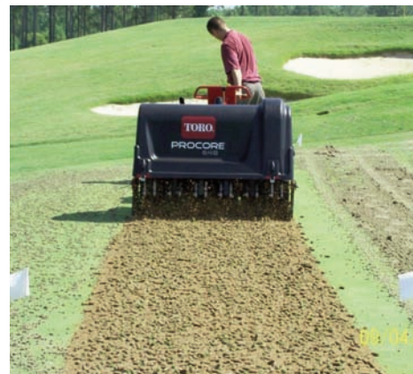
Cultivation treatments being applied on Sept 4. Left lane shows a 0.25" tine treatment; middle lane shows a 0.5" treatment; right lane shows a 0.25" coring + verticutting treatment.
