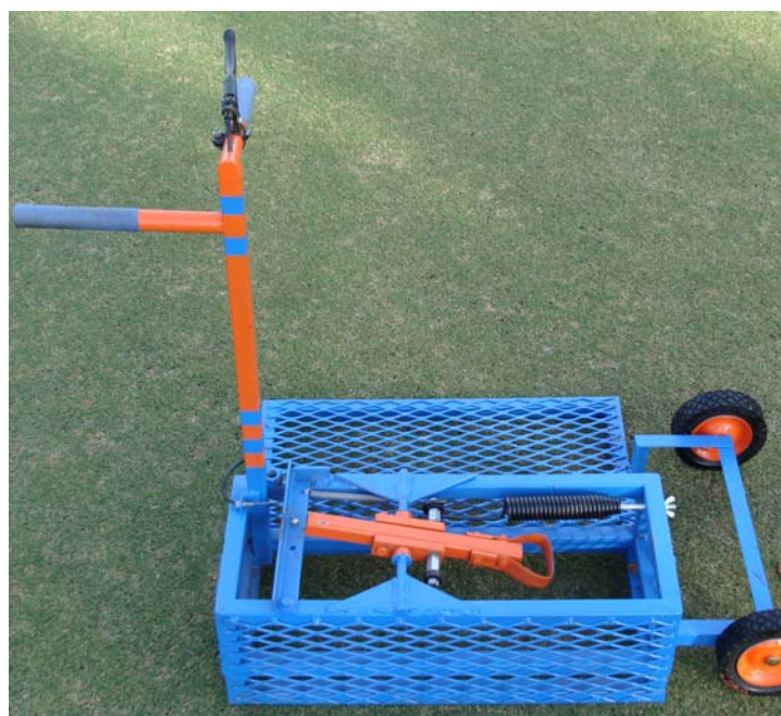
Divots are removed from the plots using a divot machine constructed from a modified clay pigeon thrower.
