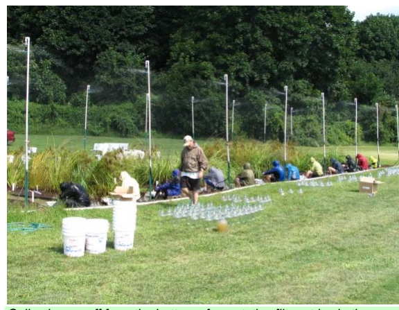
Collecting runoff from the bottom of vegetative filter strips in the presence of overhead rainfall.
