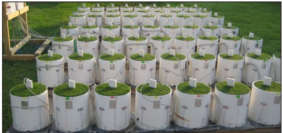
Sixty-three test columns were constructed from 332-mm (13-inch) inner diameter PVC pipe attached to a PVC sheet-lined plywood base.
