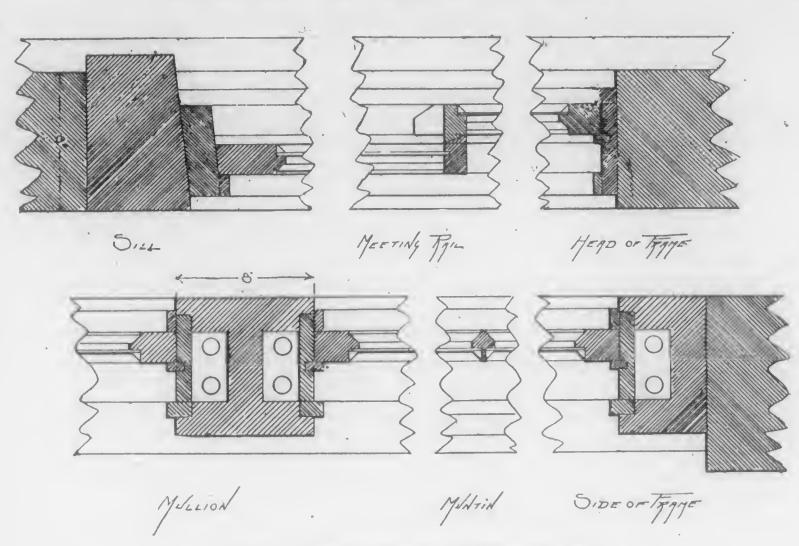
Details of Concrete Setting of Window Frames
