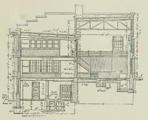
Fig. 4.-Cross-Section Through Machine Shop
