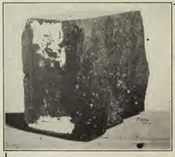
This Hall Brick was subjected to over 150,000 pounds pressure, equal to 30,000 for the Whole Brick(15,00 per square inch) absorption test thritteen one hundredth of one per cent. Test made by Engineering Department City of San Francisco.
