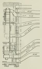
Fig. 2 .- Plan of Heaters in Main Shop
