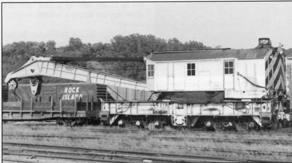
Car 900310 was seen at Council Bluffs, Iowa, on August 10, 1975. It was originally powered by oil, but was converted to diesel power in 1976. The boom and underframe were welded. Its assignments included La Grande, Ore.; Stockton, Calif.; North Platte, Neb.; Council Bluffs, Iowa, and back to Stockton, Calif. The railroad has used a wide variety of boom cars over the years. This particular car has side stakes, but is otherwise a conventional flatcar. G.R.Cockle, collection of John C. LaRue Jr.
