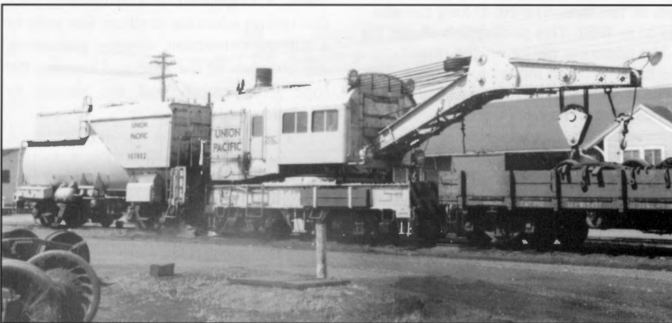
Number 900307 was a 100 ton model built in 1906 by Industrial Works. It was photographed at Grand Island, Neb., in May 1961. It was converted from coal to oil in 1953, and before it was retired in 1969, it was assigned to Albina, Ore., Yermo, Calif. and then Grand Island, Neb. Rumbolz, collection of John C. LaRue Jr.
