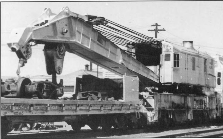
Number 903044 was photographed at Green River, Wyo., on August 7, 1966. Constructed by Bucyrus-Erie in 1945, it had a capacity of 250 tons. It weighed in at 356,800 pounds and it was 36' long. It was not self-propelled, and was originally coal-powered, but was later converted to coal in 1953 and finally to oil in 1975. It was assigned to Green River and was later sent to Las Vegas until it was retired. L. Callolia, collection of John C. LaRue Jr.
