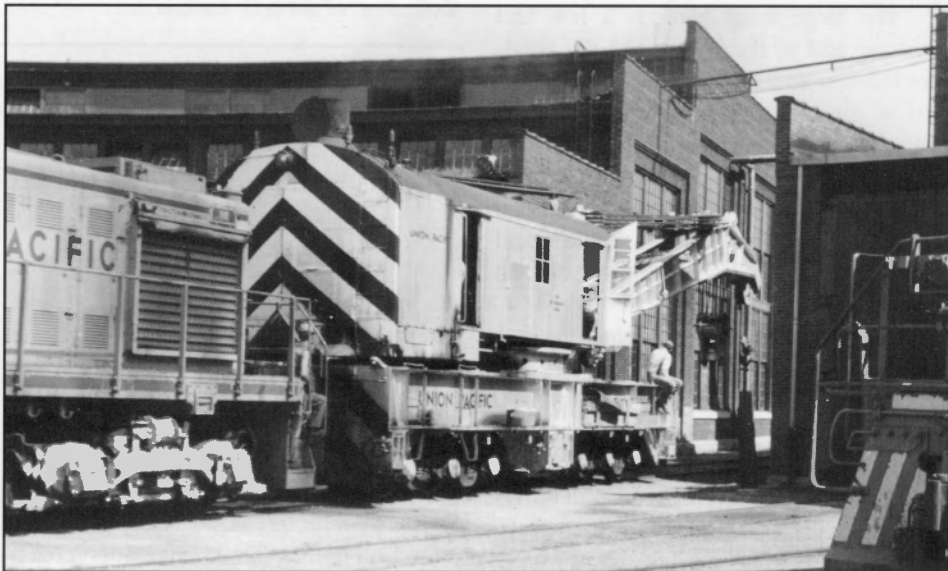
Derrick 910005 was built by Bucyrus-Erie in 1945. With a 36’ length, it had a capacity of 250 tons. Originally powered by coal, it was converted to oil in 1951, and then to diesel in 1978. The 12” black chevrons had recently been added when it was seen at the Cheyenne roundhouse in July, 1966. It was assigned to Cheyenne before being transferred to Pocatello. A.J. Wolff
