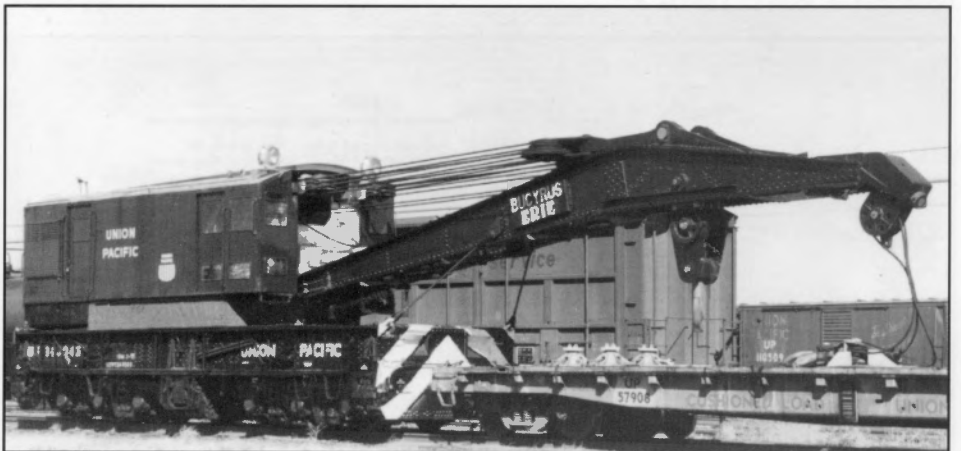
Bucyrus-Erie built 200 ton wrecker number 903043 was seen at Council Bluffs, Iowa, on February 28, 1977. It was converted from oil to diesel power in 1977 and was all-steel construction. Weighing 377,800 pounds, the car was 36' long. The boom and chassis were riveted unlike the later models from Bucyrus-Erie which were welded. Following World War II it was assigned to Las Vegas, Pocatello, and finally Ogden before it was retired. Note that the boom car was a regular Union Pacific flat car, and not a maintenance flatcar with sides to hold additional equipment needed to clear up wrecks. G.R. Cockle, Collection of John C. LaRue Jr.
