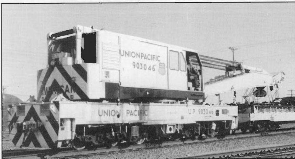
This view of 903046 shows the massive frame and body needed to be able to lift 250 tons of railroad equipment. The end of the car was aluminum colored with 12 inch black chevron stripes for visibility, and the two three-axle Buckeye trucks span almost the entire length of the car body. It was photographed at Cheyenne in 1985, along with its boom car, which was made from a retired heavyweight passenger car.
