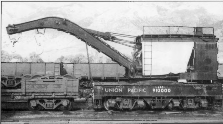
A side view of 910000, built for the Los Angeles & Salt Lake in 1904 by Industrial Works. The 60 ton crane had an open cab, which was protected by canvas when not in service. The short, 24-foot-2-inch frame seems small compared with today's 250 ton wrecker. Following World War II this wrecking derrick was assigned to Lynndyl and Provo, both in Utah, until its retirement in the late 1960s. This view was taken at Provo, Utah, on October 3, 1966. H.N. Proctor, J.C. LaRue collection
