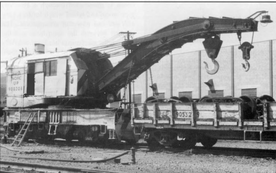
UP 900308 was assigned to Huntington, Ore., when this photograph was taken on August 16, 1967. With a capacity of 120 tons, the car was built in 1910 for the Oregon-Washington Railroad and Navigation Company by Industrial Works. It was converted from coal to oil power in 1953, and finally retired in 1976. The cylinders on this wrecker were boxed in with a sheet metal cover. W. Pennington, Collection of John C. LaRue Jr.
