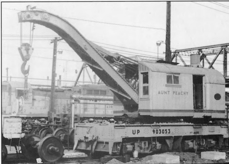
Aunt Peachy, presumably not the official Union Pacific designation for wrecking derrick 903053, was photographed at Denver on December 20, 1969. This piece of equipment was built in 1901 by Industrial Works for the Union Pacific. The 40-ton crane was 24'2" long, and weighed 149,000 pounds. It burned coal, and also had a steel underframe with a wood superstructure. Originally numbered 02800, it was changed to 03053 in 1918, and to 903053 in the 1959 renumbering. It was assigned to Denver for almost 70 years until it was donated to the Forney Transportation Museum in Denver. F.H. Worsfield, collection of John C. LaRue Jr.
