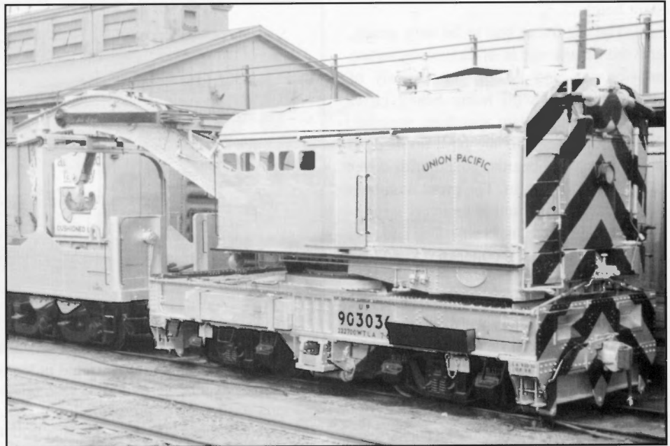
UP 903036 was a 120 ton Industrial Brownhoist. A handrail had been added to the top of the cab. Minor variations can be noted in the painting and lettering with all the wreckers. The Los Angeles wrecker had black trucks, boom rods and tool crib. F.H. Worsfield, Collection of John C. LaRue Jr.
