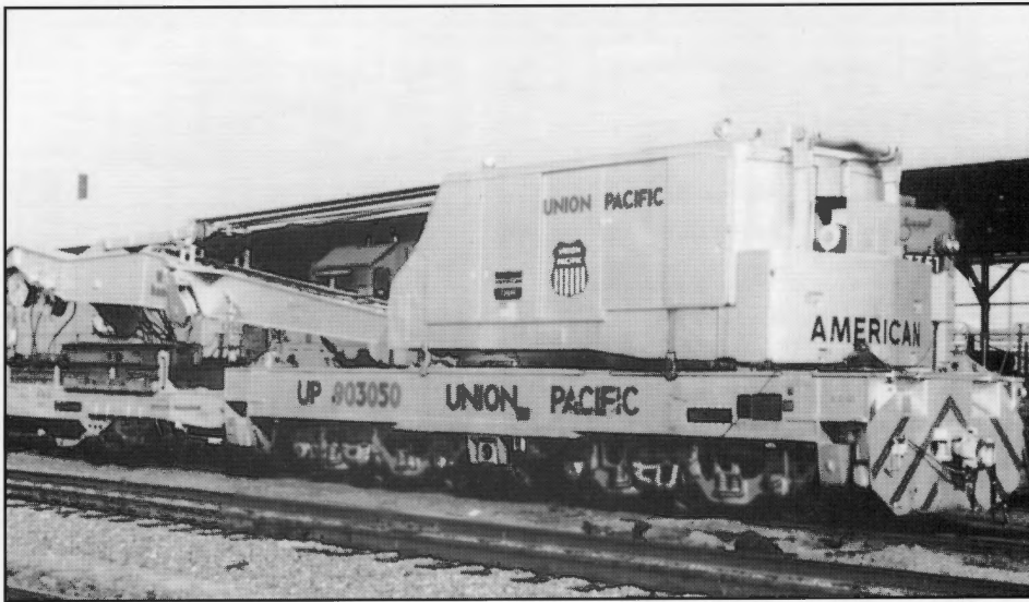
Union Pacific wrecking derrick 903050 was one of the last, if not the last built for the railroad. Constructed in 1973 by American Hoist & Derrick, it has a capacity of 250 tons and is diesel powered. It is self-propelled and has roller bearing equipped Buckeye trucks. It is assigned to Hinkle, and was photographed there on September 26, 1978. The standard paint for the American Hoist & Derrick cars is aluminum with black lettering without the 12-inch chevrons. J.R. Quinn, collection of John C. LaRue Jr.
