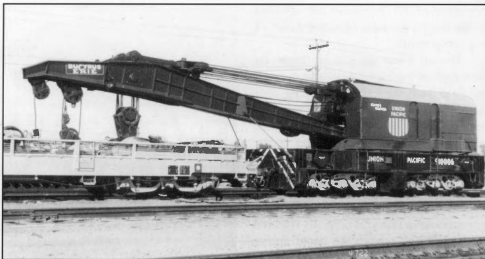
Number 910006 was photographed at North Platte, Neb., on Dec. 17, 1978. The self-propelled, diesel powered model was built in 1956 by Bucyrus-Erie. It had a capacity of 250 tons, with roller bearings on the trucks. The standard paint scheme for the B-E cars was dark (Batavia) green body, black underframe and trucks, white lettering, aluminum roof, and 12” chevron black and white stripes, front and back. The stripes were not standard when this photograph was taken. The derrick was originally assigned to Council Bluffs before being moved to North Platte. G.R. Cockle, J.C. La Rue Collection
