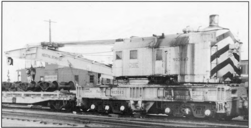
Wrecking derrick 903042 was assigned to Rawlins, Wyo., when photographed on September 3, 1970. Built by Industrial Brownhoist Corporation in 1926, the 200 ton wrecking derrick weighed 345,100 pounds and was 36'4" long. It was converted from oil to diesel in 1978, and was self-propelled. Note the black stripes on the end. The frames of these cars are basically massive I-beams, with heavy riveting and stiffeners to make them strong enough to lift and move heavy equipment. Following World War II this wrecking derrick was assigned to many locations, including La Grande, Ore.; Las Vegas, Nev.; Council Bluffs, Iowa; Rawlins, Wyo.; and Kansas City, Mo.; before it was retired. F.H. Worsfield, collection of John C. LaRue Jr.
