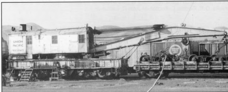
No. 903043, was photographed at Pocatello on September 12, 1969. The rear end of the unit was the counter-weight and scrap metal was typically placed in it. Note that the boomcar is holding some spare trucks. F.H. Worsfield, collection of John C. LaRue Jr.
