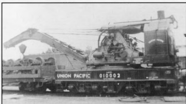
120- ton 902005 was built for the Oregon Short Line by Bay City in 1913. Converted from coal to oil in 1952, it had plain bearings and was not self-propelled. Before retiring in 1975, it was assigned to Glens Ferry, Idaho and Albina and Hinkle, Ore. When this picture was taken at Omaha on June 26, 1975, it had just returned from clearing up a wreck, as evidenced by the engine hood on the boomcar. The walkway on the roof was constructed from GP 9 handrails J.R. Quinn, collection of John C. LaRue Jr.
