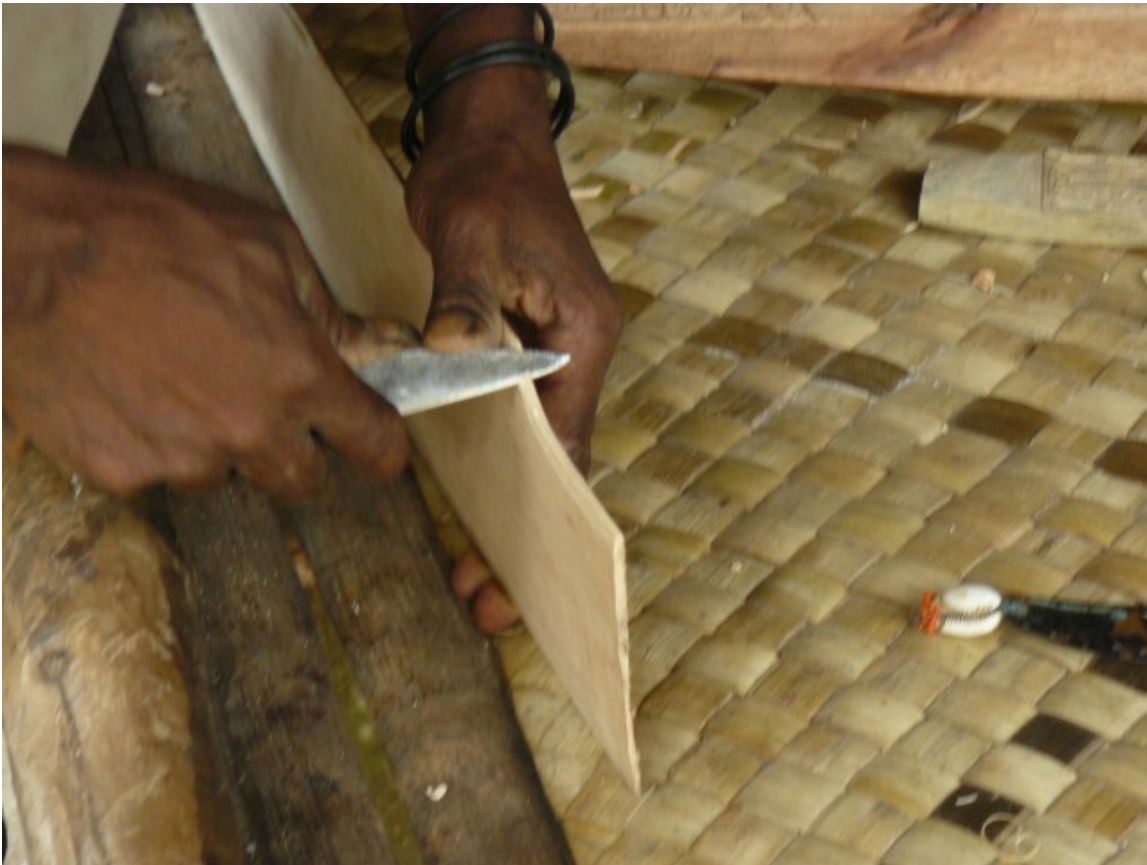
From the 2012 model anageg: trimming a cut-away on the bottom end of the bottom strake which must fit into the groove (atonen) designed for it towards the end of the keel. Hours must be devoted to cutting a log into a strake then more time with an adze so that it is about ready; then even more time for the final stages of fitting.
