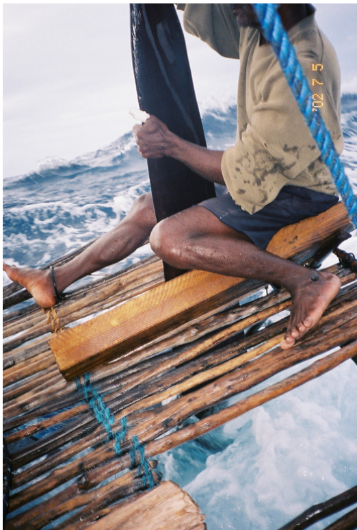
Withdrawing the kavavis (rudder) as a wave rolls into the outrigger.
