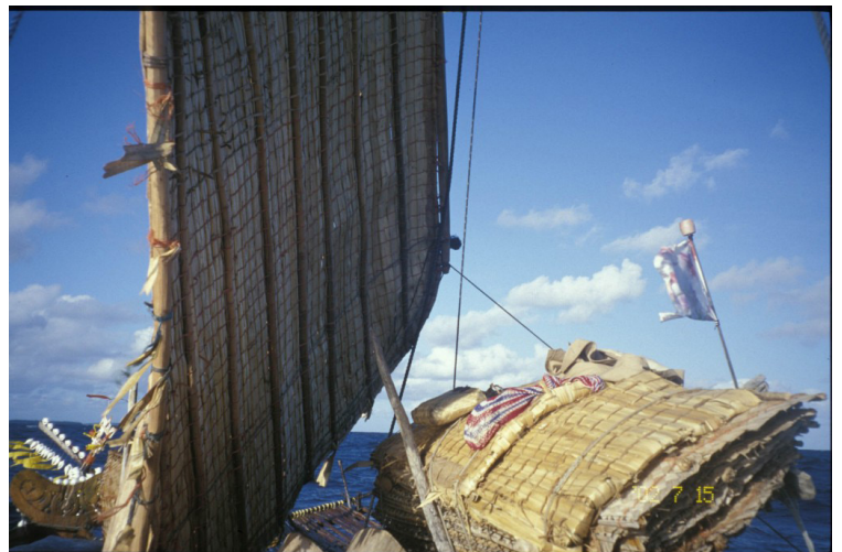
Levanay sailing into the wind. The sailing direction is straight through the prowboard at the lower left corner of the frame. The rough, slatted inside of the sail centers the scene; Chapter 5 describes the sail structure. To the upper right is the flag, blowing into the camera. Below it is the rack of woven coconut fronds used to protect the sail when it is stored; on top of the fronds are the remains of the craft’s previous sail.
