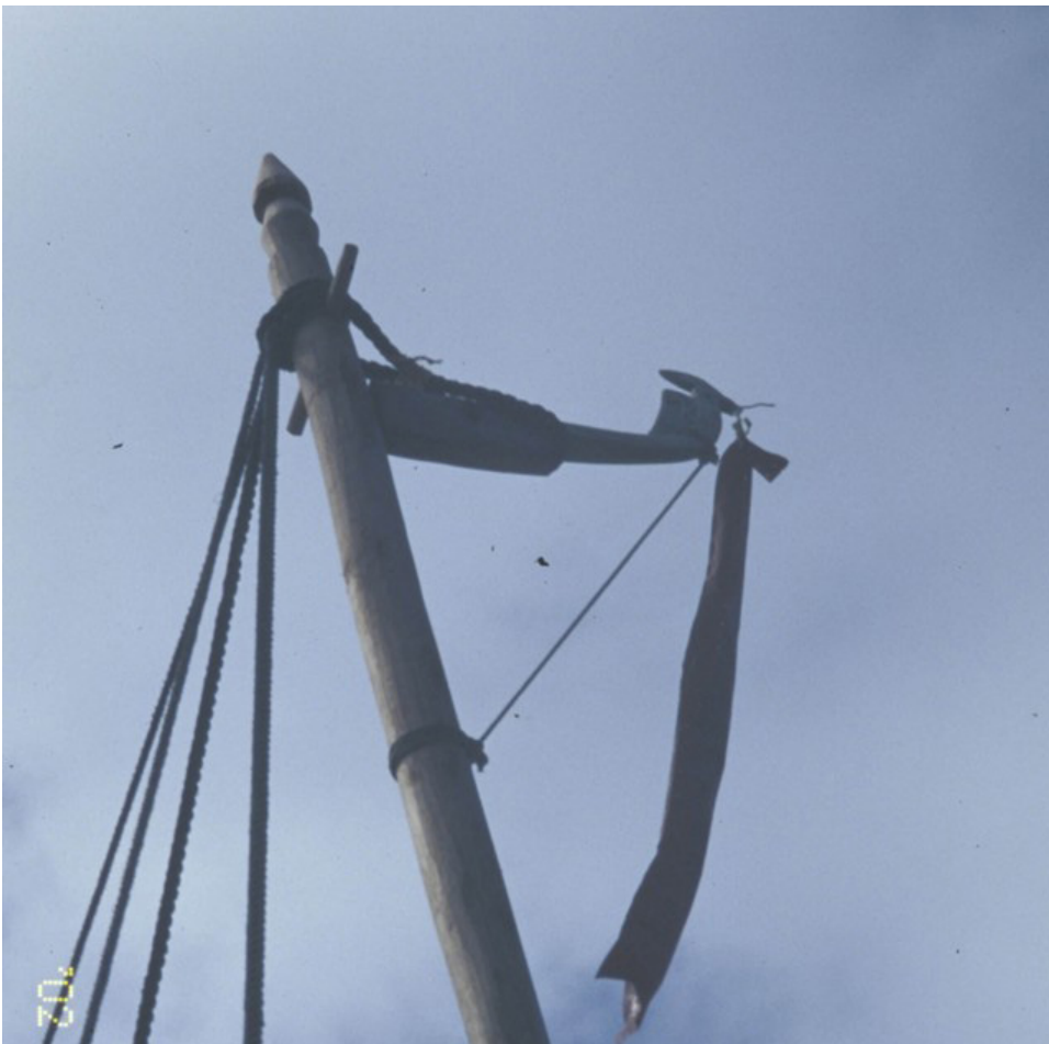
From 2002, balau lines looped around top of Lavanay's new mast while in Nasikwabw. The sipbalau knot is named from this line. The placement of three sipbalau knots, one at the top of the mast, two on the outrigger platform, controls the degree to which the mast arcs toward the outrigger float and pivots more or less to the leading direction of the craft.
