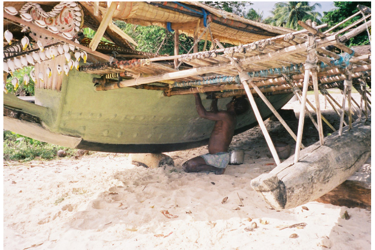
“Painting” Levanay with seaweed. Note that the forward cross beam is not caulked.
