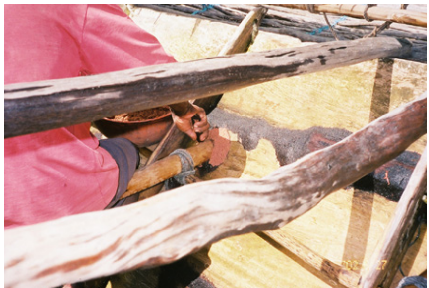
Caulking a cross beam inside the Levanay's hull.
