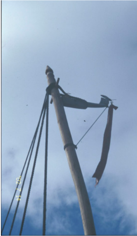
Left: From 2002: Distant shot of Lavanay's new Nasikwabw mast showing the balau and powan balau. Although people speak as if there is just one balau line, there are usually two said to be in a mother/child relationship, the latter helping the former. 2002R4Mast
