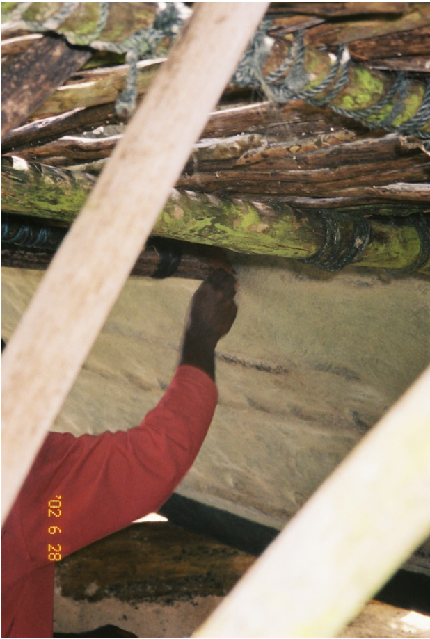
Caulking a cross beam under the outrigger platform.
