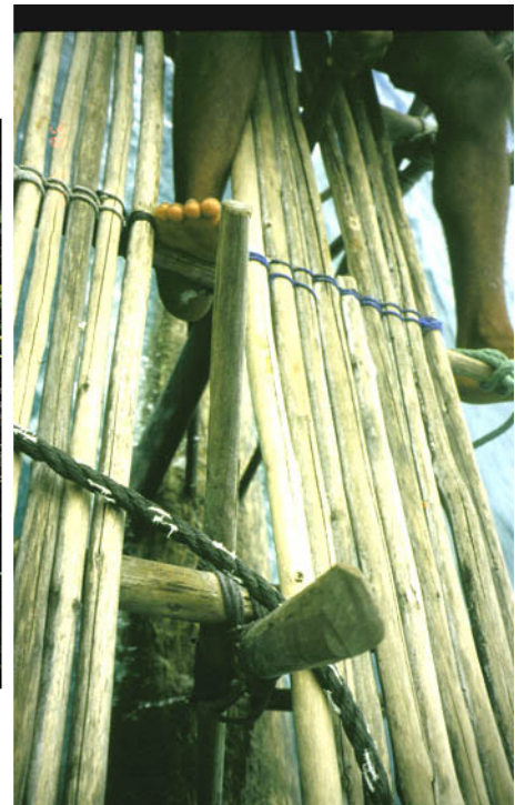
Left: From 1998, a Nasikwabw anage showing the gap on the platform designed for the insertion of a kavavis. The kavavis goes up and down against the outrigger float, pressure from the water pushing the piece into the float. The large gap to the very left is a toilet.
