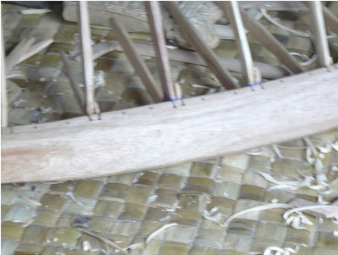
2012. From the model anageg the central structure of the keel shows how pairs of gulumom (rib) are tied into place. The holes between the ribs are for tying the bottom strake.
