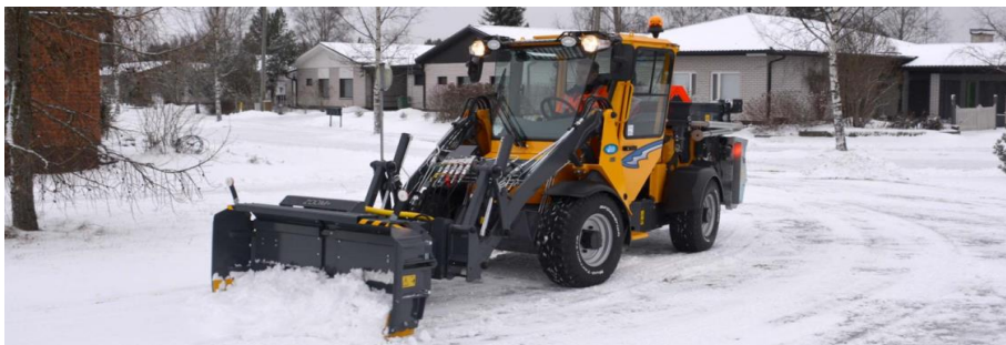
A multifunctional equipment equipped with snow removal accessories and equipment and for road maintenance during summer.
