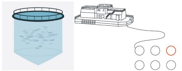
FIGURE 3.12. An aquaculture facility is usually made up of multiple net pens (left), which are connected to a feed barge (right). These are permanently moored at the site. *Source: Mowi / Nova Sea*<sup>323</sup>
