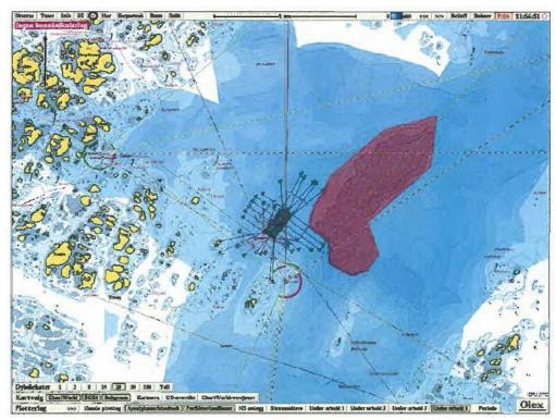
FIGURE 3.23. Plan showing the proposed moorings of the facility at Hysvær in relation to the adjacent shrimp field (red), which lies over the deeper area of the site. *Source: Nova Sea*<sup>344</sup>
