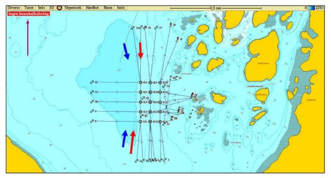
FIGURE 3.17. This plan shows the details of the proposed location of the aquaculture facility at Rørskjæran and the position of its moorings. *Source: Mowi*<sup>330</sup>
