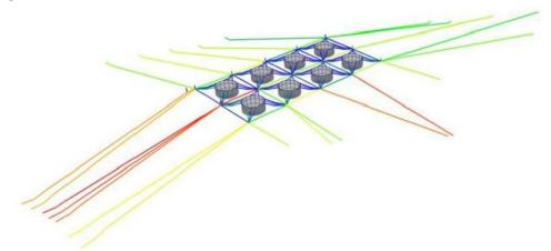
FIGURE 3.11. Modelling of the mooring system for the net pens that would make up the proposed facility at Rørskjæran. *Source: Mowi*<sup>321</sup>
