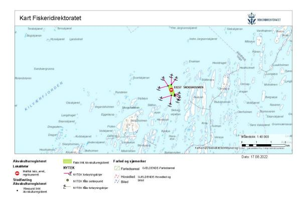
FIGURE 3.32. The layout of the facility at Skogsholmen showing its mooring system. Source: Fiskeridirektoratet
