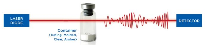
Figure 1: Non-destructive headspace analysis using a laser diode that shines through the headspace of a container. Oxygen, carbon dioxide, moisture, and pressure can be measured in the headspace of parenteral containers.
