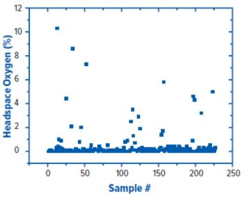
Figure 4: Headspace oxygen content of vials located in zones 1-3. Vials in these locations show air ingress due to stopper pop-up.
