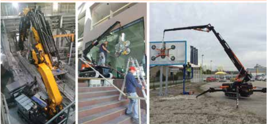
M060: PICK AND CARRY - Max hydraulic outreach: m 3 – Max load capacity Kg 240 – Width mm 780
