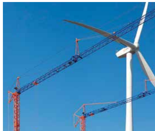
Arcomet's new crane has 8,000kg capacity, a 50 metre jib and maximum 36 metre hook height.
