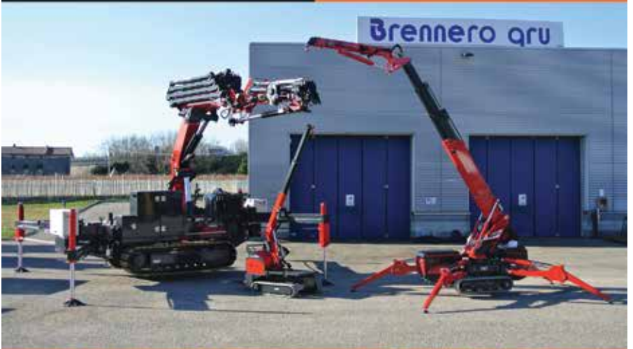
CWE 525: Max hydraulic outreach: m 30 Load capacity Kg 14500 – Easy access: Max width mm 1850 M250: Full hydraulic JIB with 195° opening Max hydraulic outreach m 15.65
