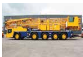
LIEBHERR - MK100/110 Tower Cranes 8t, 52m Flight 68m Lift Height, Intarder 2006 | PHM-Id 08998
