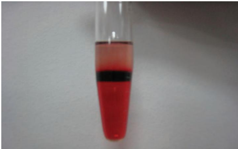
Fig. 6. The blood sample (diluted \frac{1}{2} with RPMI) after Percoll gradient separation, 1.130 (20°C-2500rpm, 20 minutes)
