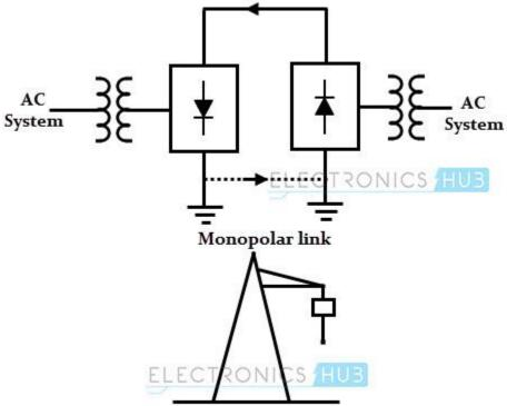
Monopolar HVDC links were used only for low power rating and mainly for cable transmission. In some cases the monopolar lines installed earlier are converted into bipolar systems by adding additional substation pole and transmission pole.
