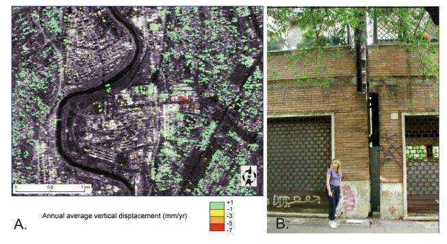
A. Estimate of vertical displacement of building from multi-image radar map analysis (from Giordano, Mazza et al., 2004). At present, several edifices built over unconsolidated clays are monitored from selective subsidence. This image is a courtesy of F. Ferrucci and has been obtained by comparing 10 years of satellite images. B. Evidence of differential subsidence on the structure of buildings.
