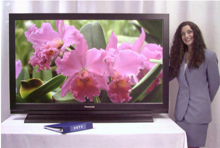
Figure 1.1 A 60 inch diagonal color plasma display panel. The display has an array of 1366 \times 768 full color pixels, and a total viewing area of 1328 \times 747 mm. It weighs 75kg and has a 5 inch thickness.
