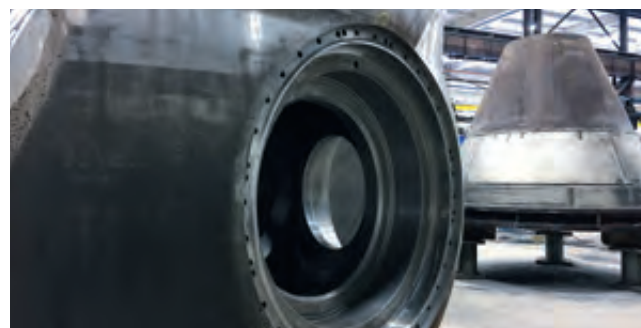
Due for an overhaul after 30 years: parts from Voith Hydro Kaplan turbines in York.
