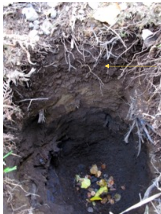
Layer of sand and gravel
