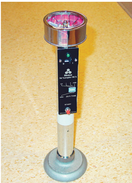
RCS-sampler (Reuter Centrifugal Sampler).
