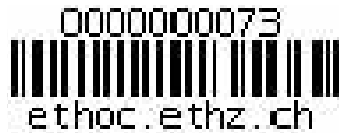
Figure 7.1.: Picture of a printed ETHOC code with unique ID 0000000073 displayed both in human-readable form and in barcode representation, together with the former URL of the ETHOC Web portal at ETH Zurich
