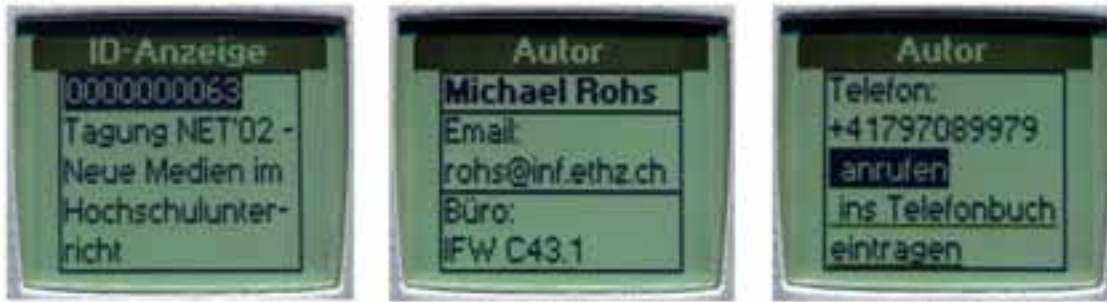
Figure 7.3.: On the mobile phone, a WML page is shown as the result of scanning a paper document
