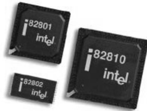
Figure 4.32 Intel 810 chipset showing the 82810 (GMCH), 82801 (ICH), and 82802 (FWH) chips. Photograph used by permission of Intel Corporation.
