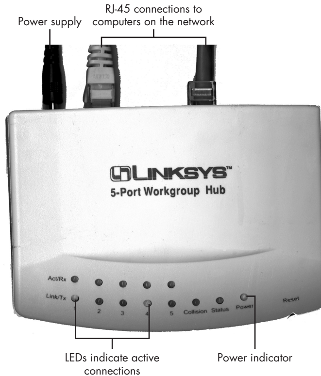
Figure 19.14 A typical 10BaseT five-port workgroup hub. Connectors 1 and 4 are connected to computers (as shown by the lights at the front of the hub (bottom of the picture)). The light at right indicates the hub is receiving power from a AC/DC transformer “brick.”
