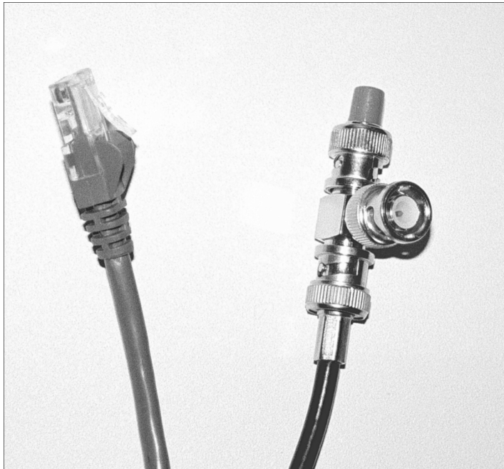
Figure 19.6 An RJ-45 UTP cable (left) and a Thin Ethernet cable with BNC T-adapter and terminator (right).
