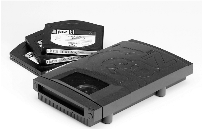
Figure 12.6 A 2GB external Jaz drive and media. Photo courtesy Iomega Corporation.
