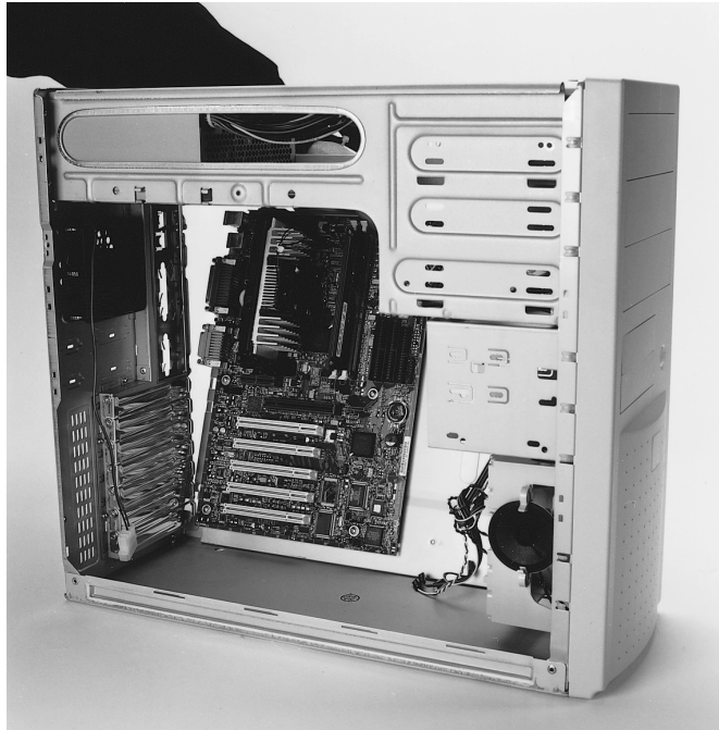
Figure 24.13 Installing the motherboard and tray into the chassis. Case courtesy of PC Power & Cooling, Inc. Motherboard courtesy of Intel Corporation.
