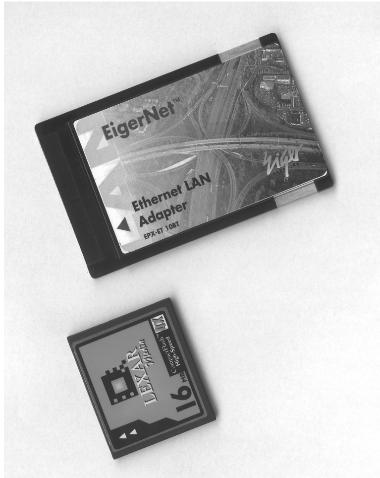
Figure 12.11 A Type II PC Card (top) dwarfs a 16MB CompactFlash card (bottom). The “4x” designation on the CompactFlash card indicates that the card transfers data four times faster than a standard model.
