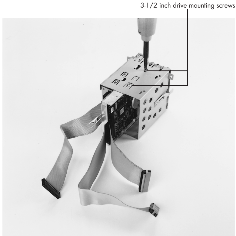
Figure 24.23 Use four screws to secure each drive to the drive cage. Chassis courtesy of PC Power & Cooling, Inc. Hard drive supplied by Micro X-Press.
