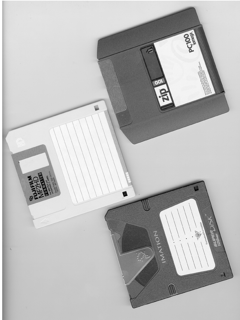
Figure 12.2 The Zip 100MB disk (top) compared to the standard 3.5-inch 1.44MB diskette (middle) and the LS-120 SuperDisk (bottom). The Zip disk is thicker, has a tapered top, and has a much narrower shutter than either the LS-120 or 1.44MB diskettes.
