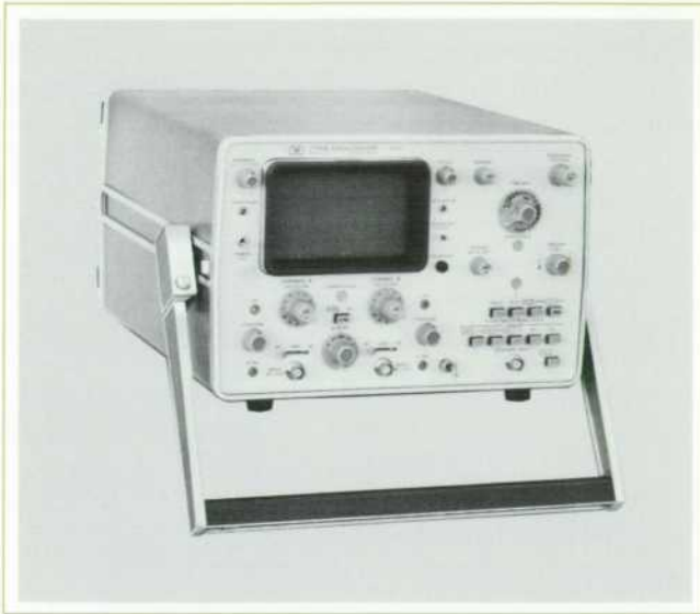
Fig. 6. Lower cost Model 1700A, for certain communications applications and others not requiring delayed sweep, has same 35 MHz vertical amplifier and 10 ns/div main sweep performance as Model 1701A, but omits delayed sweep.
