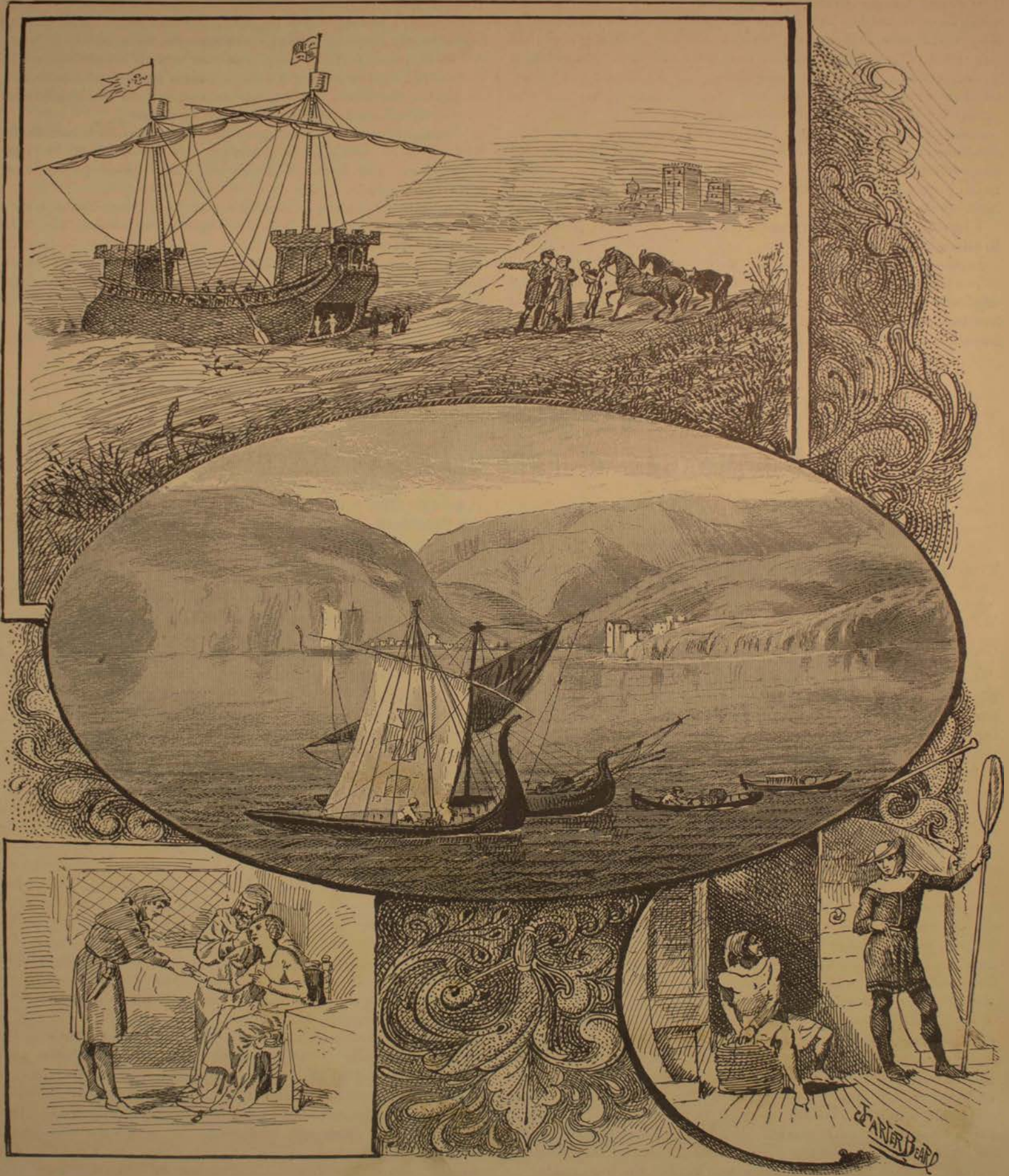
1. Curious ship of the 14th century, showing castle in the bow, from which comes our name for that part of a vessel, "forecastle": and also showing how the stern was opened to receive freight and passengers. 2. Machico. 3. Costumes of the 14th century. 4. Sailors of that period.
