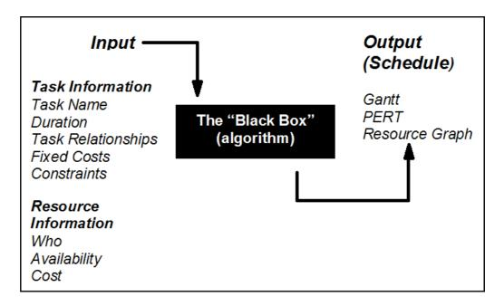
Figure 2-4: The Input/Output Model
