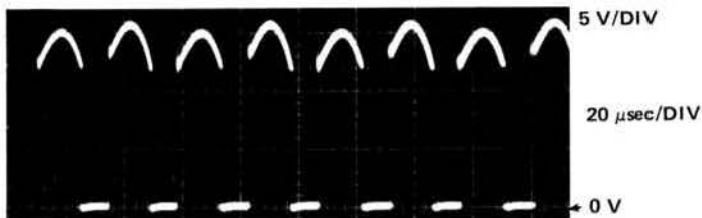
K.) At collector of Q1900 during normal operation.
