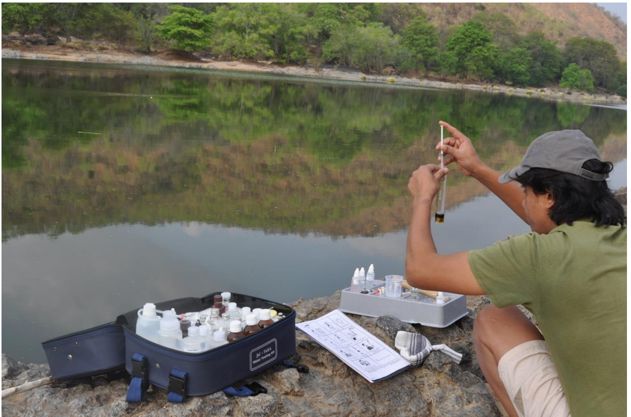
Fig 9. WASI volunteer conducting a test for dissolved oxygen at the crocodile rock pool.
