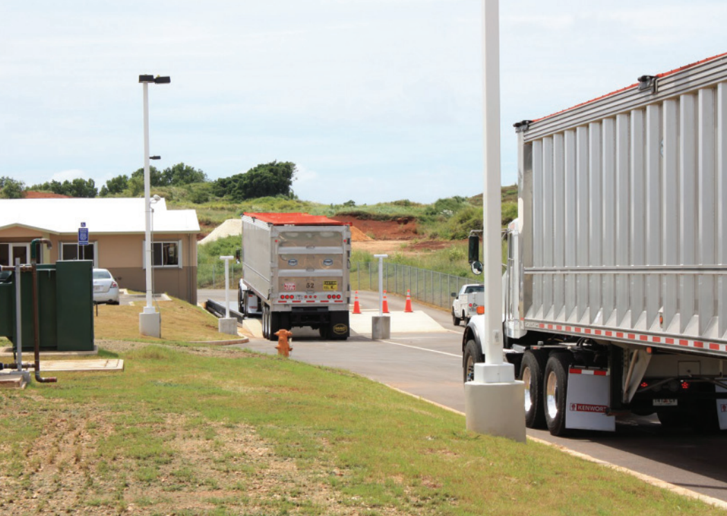
Trash trucks cross the weigh scales to deliver waste to the Layon Landfill. When the Receiver arrived, there were no scales at the Ordot Dump, which closed on August 31, 2011.
