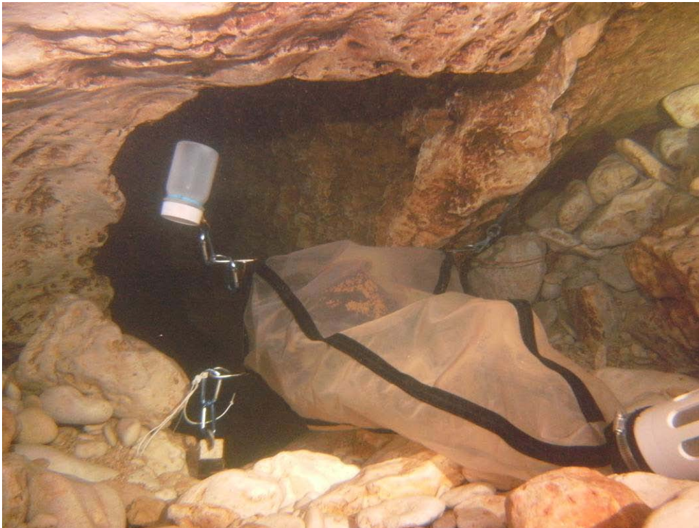
Figure 6. Drift net set up at the constriction in Jacobs Well. During this low flow regime the drift net is flaccid.
