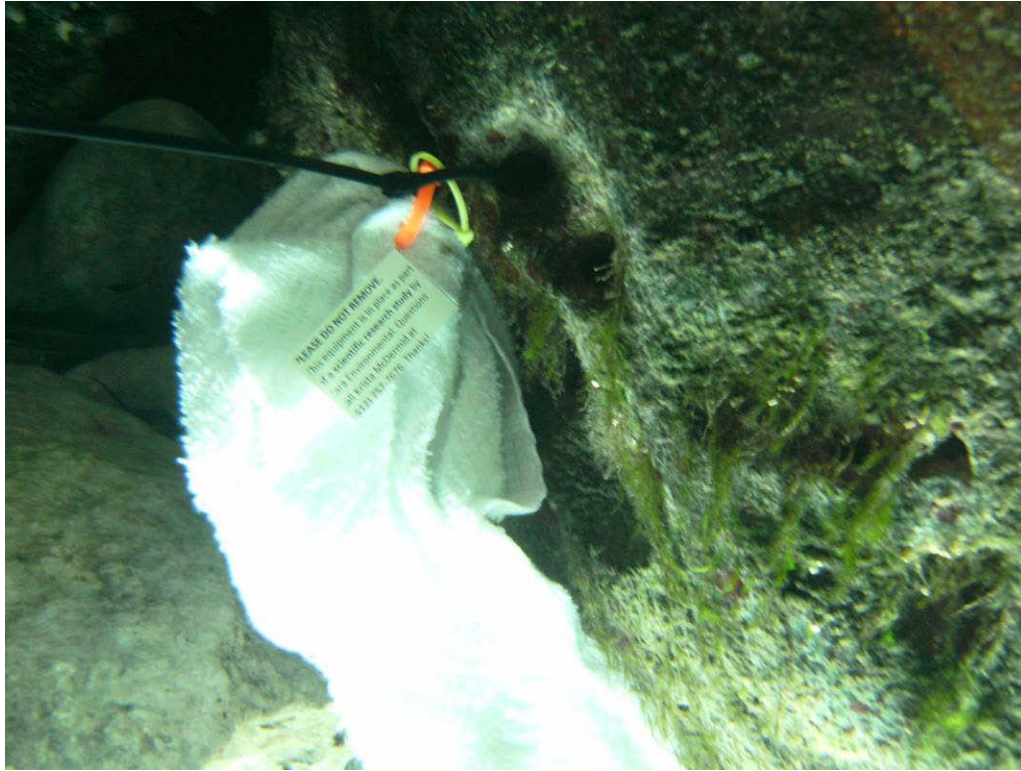
Figure 3. Cloth lure secured to the side of the cave shaft in Jacobs Well.
